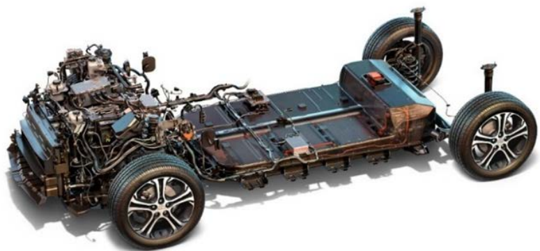
Current electric vehicle (EV) platform (GM's 2017 Chevrolet Bolt battery-electric vehicle chassis with electric powertrain)
