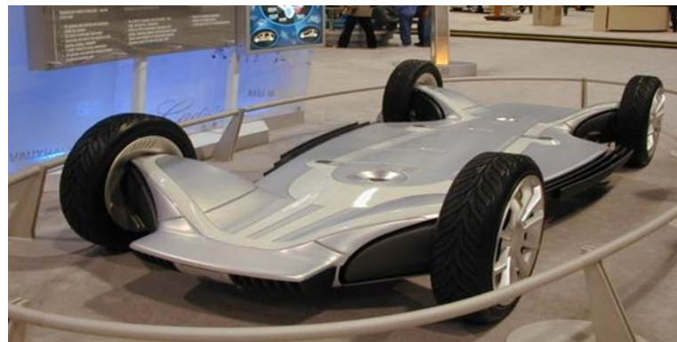
Future skateboard platform design concept (GM's flat skateboard chassis containing electric powertrain)
