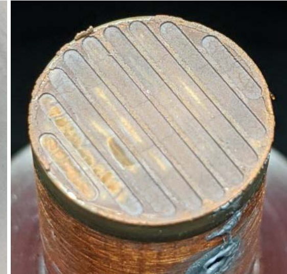
After test: Noticeable oxidation/deposits
