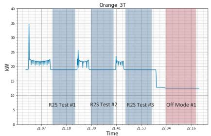
Ready-to-scan test was repeated 3 times with different preceding active scanning protocols to determine if it is affected by the power draw.
