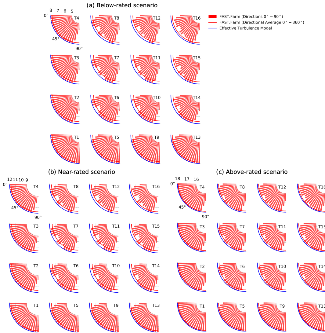
Figure 13. Mean hub-height wind speed ( \text{m s}^{-1} ) at each wind turbine in the farm for each wind speed scenario. The FAST.Farm bars represent seed-averaged results for wind directions 0^{\circ} – 90^{\circ} , while the solid line is the directional average for wind directions 0^{\circ} – 360^{\circ} . The effective turbulence model (EFF) line is constant for all subplots due to the lack of wake wind speed deficits in the EFF modeling approach.
