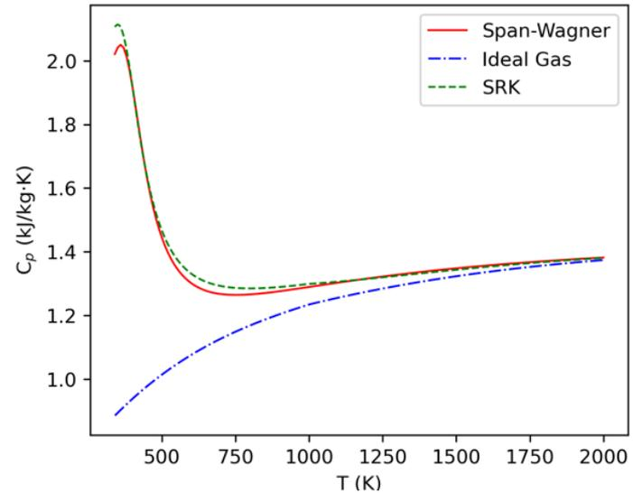
Specific heat vs. temperature at 303.9 bar
