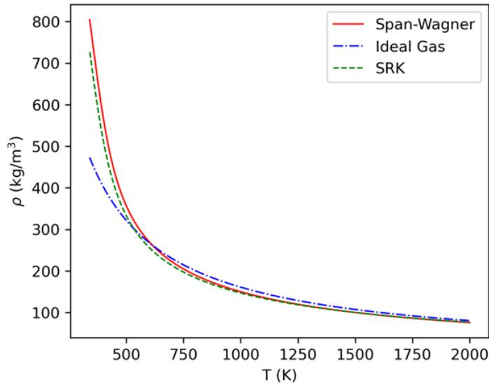
Density vs. temperature at 303.9 bar
