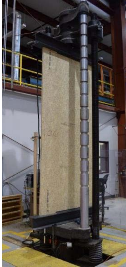
Figure 8. ASTM E72 axial load compression buckling test setup using Home Innovation Research Labs' UTM
