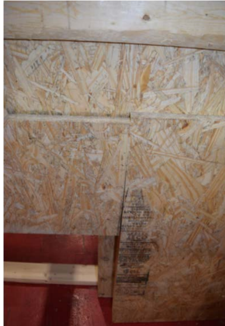
Figure A-15. Test 3 panel joint slip of inner panel splice at end of header
