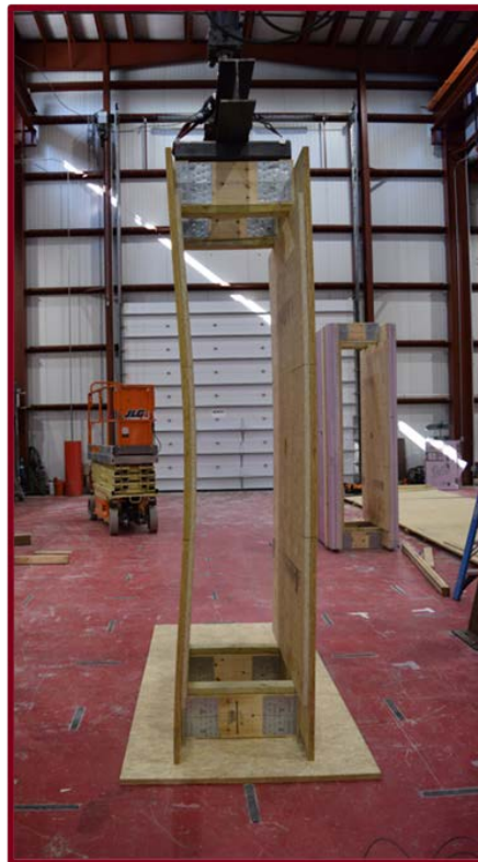
Figure D-1. Axial load test apparatus
