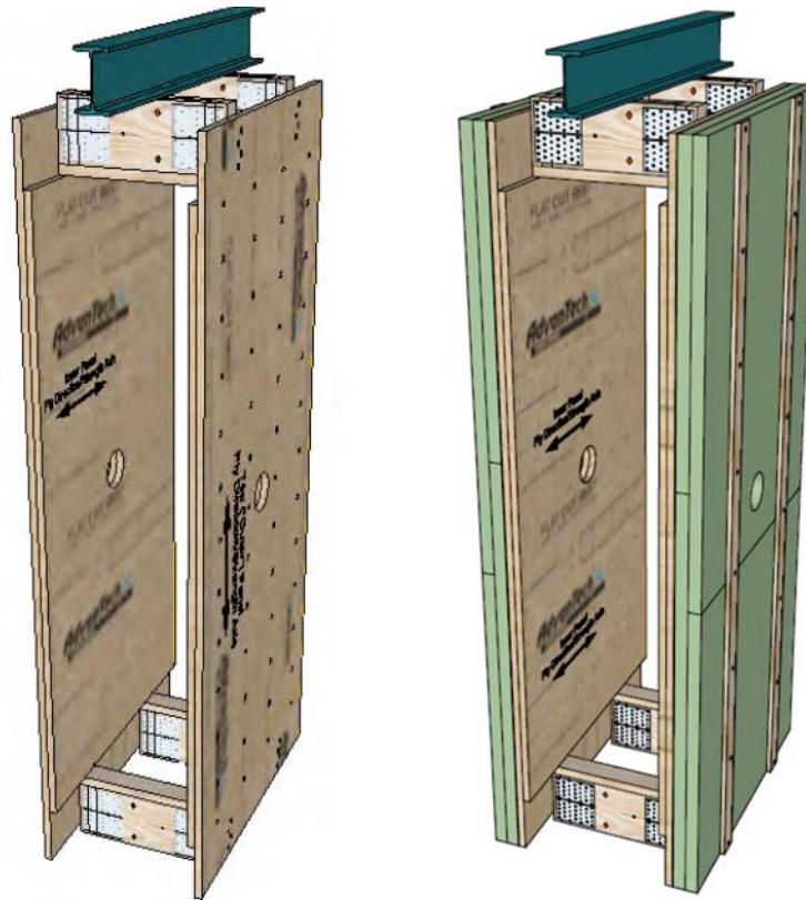
Figure D-2. Test specimen drawings for axial with fixity
