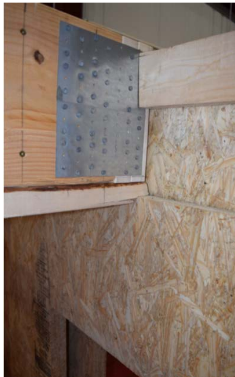
Figure A-16. Test 3 connection failure of joint truss
