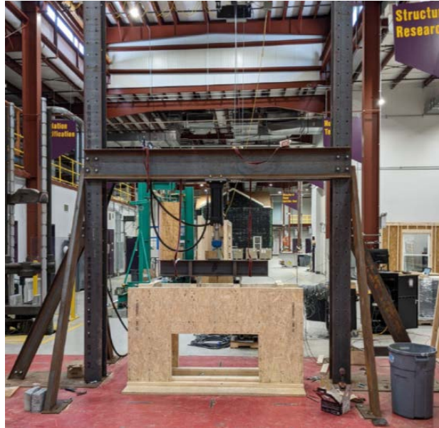
Figure A-1. SPS header test apparatus
