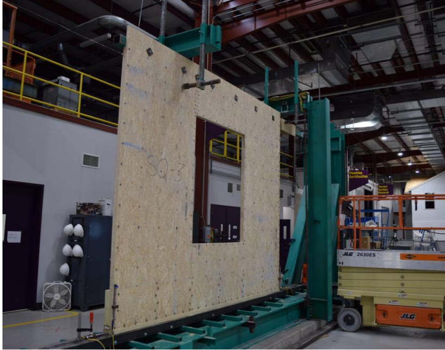
Figure 11. Shear wall test apparatus and example test specimen of cross-laminated 2-ply SPS wall assembly with a window opening
