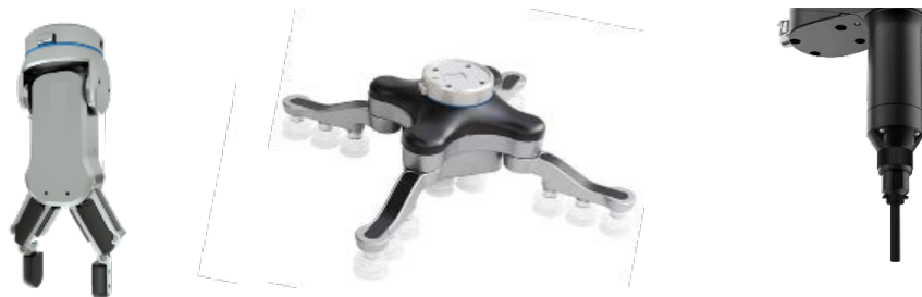
Figure 4: [Left to Right] Two-finger Gripper, Electric Vacuum Suction Gripper, and Screwdriver end-effector.
