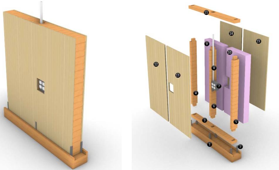
Figure 3: [Left] Render and [Right] Exploded 3D of prototype wall assembly designed for robotic assembly testing.
