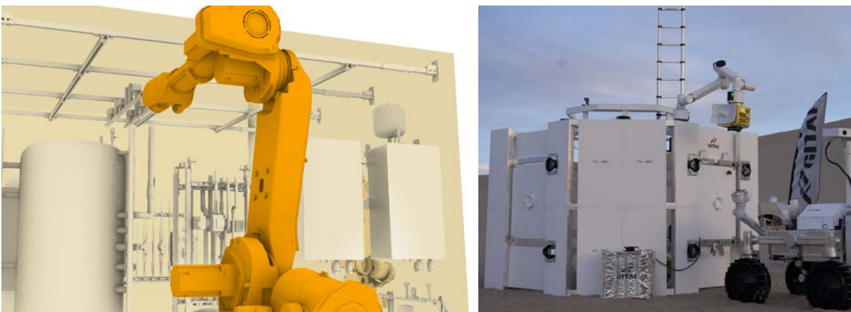
Figure 15: [Left] Ongoing research simulating robotics for terrestrial building systems integration at NREL (Muthumanickam et al., 2022); [Right] Recent robotics for lunar construction demonstration by GITAI (Nakanose et al., 2023).
