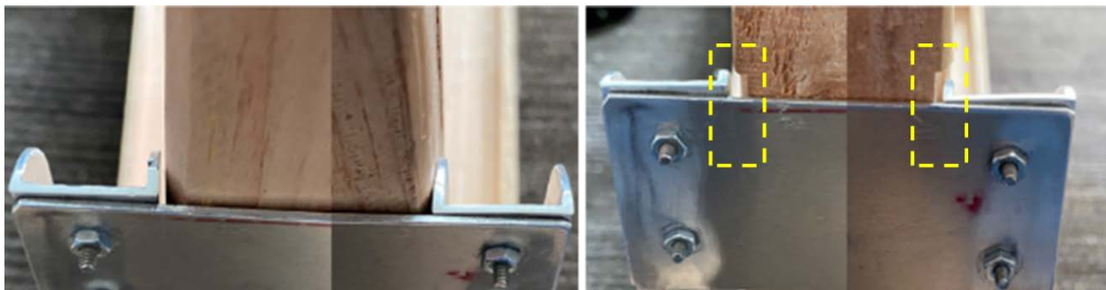
Figure 10: [Left] Stud without milled sides brushing against Aluminum C-Channel and (Right) Stud with milled sides to seamlessly slide in place between the Aluminum C-Channels
