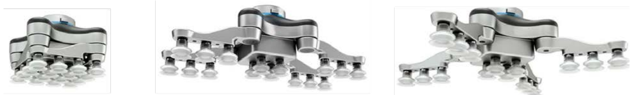
Figure 12: [Left to Right] Compact, partially expanded, and fully expanded configurations of the electric Vacuum Suction Gripper End Effector.
