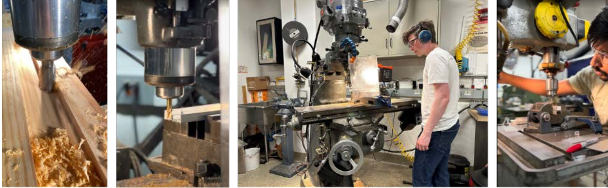
Figure 7: [Left to Right] Milling of wood and metal using Knee Mill, 3-axis Knee Mill setup, Aluminum C-Channel Cutting and Drilling
