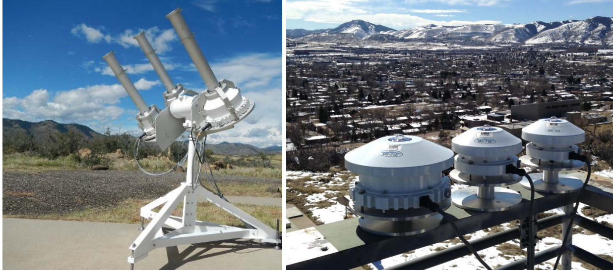
Figure 5-2. (Left) Three field spectroradiometers mounted on a solar tracker to sense the direct normal spectrum. (Right) The same three spectroradiometers mounted horizontally to sense the global horizontal spectrum.
