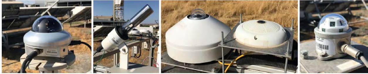
Figure 3-16. Alternative radiometers to derive DNI or DHI without a solar tracker (from left to right): Delta-T SPN1, EKO MS-90, PyranoCam (all-sky imager plus CMP21 pyranometer [Blum et al. 2022]), and Sunto Technology CaptPro.
