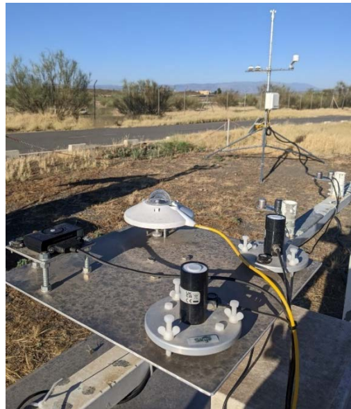
Figure 5-10. Various instruments for agrivoltaic applications. Foreground, from left to right: PAR spectrometer, pyranometer, six UV and PAR sensors. Background: wind mast with pyranometer, relative humidity and wind sensors.
