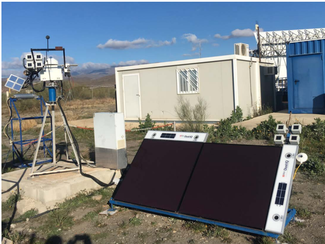
Figure 5-7. Several cleanliness measurement options for PV and CSP
