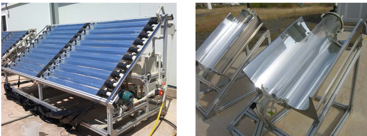
Figure 11-16. Compound parabolic collector photoreactors installed at Plataforma Solar de Almería for solar water disinfection and phytopathogen elimination from wastewater applications: (left) compound parabolic collector and (right) phytopathogen elimination system
