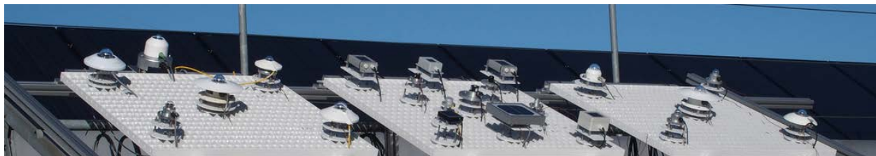
Figure 3-21. Test facility to quantify PV reference cell characteristics and compare them with other types of radiometers.
