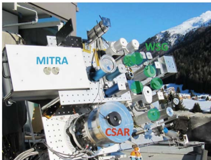
Figure 3-5. The World Standard Group of ACRs (marked in green) used to define the WRR or DNI measurement standard.
