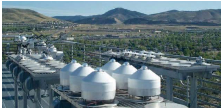
Figure 3-8. Kipp & Zonen model CM22 pyranometers installed in ventilated CV2 enclosures.
