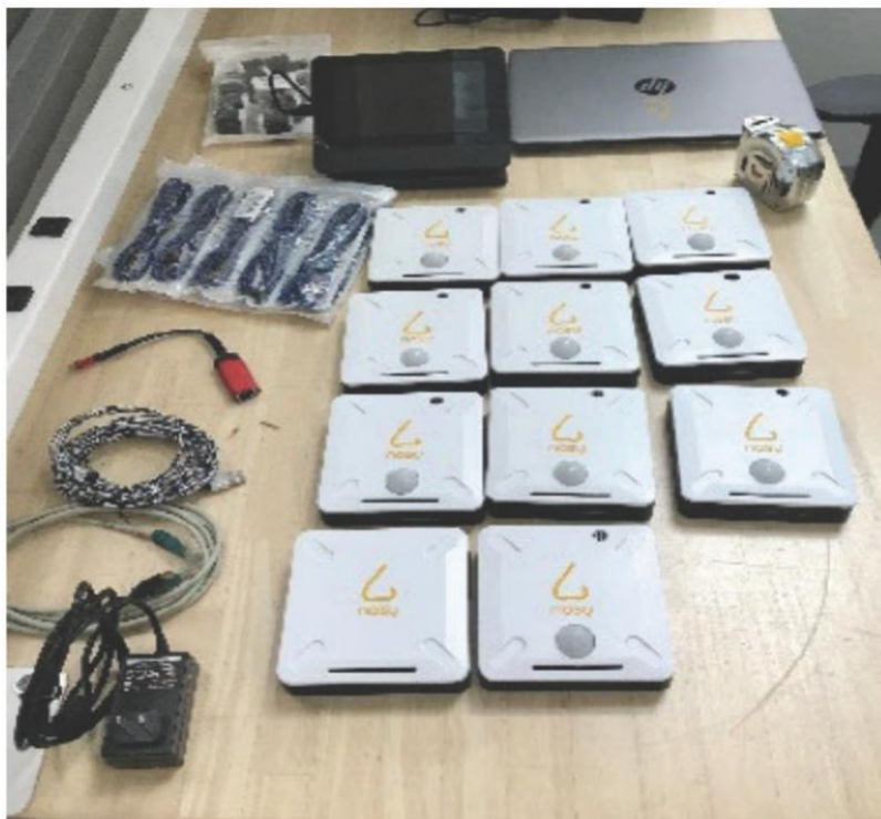
Figure 3. A photograph of the prototype sensor units and touchscreen gateway prior to installation. Each sensor has dimensions of 4"x4"x2". (Image Credit: Amanda Kirkeby, NREL)
