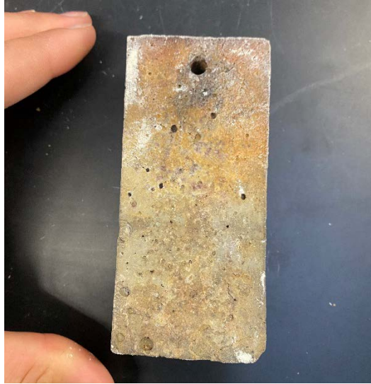
Figure 60. Appearance of a geopolymer block sample after 27 days of molten chloride salt immersion at 650°C
