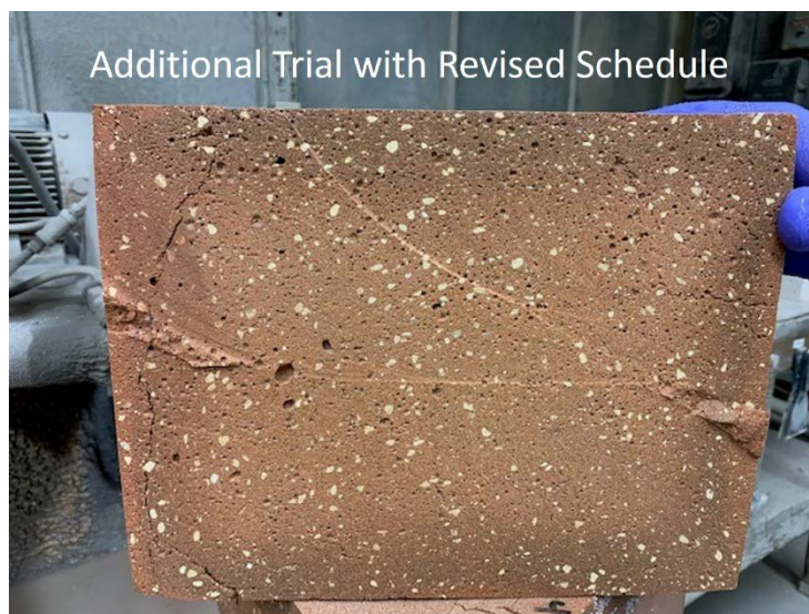
Figure 79. Cross section of a firing trial with the revised heating schedule showing minimum internal cracking
