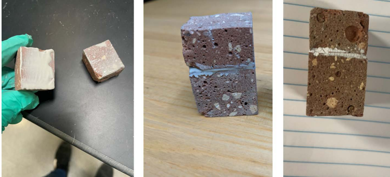
Figure 18. A geopolymer mortar joint during mortar application (left), shortly after mortar application (middle), and after 720°C heat treatment (right)
