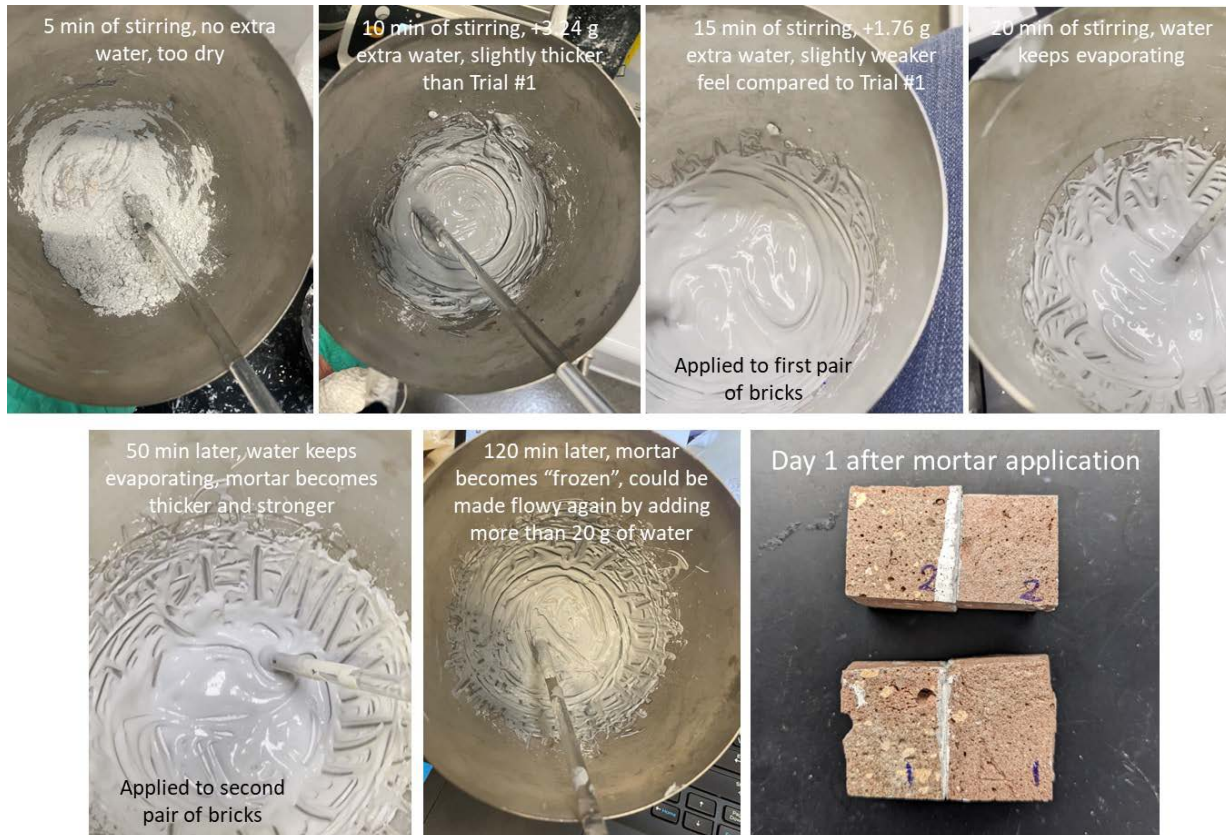
Figure 19. Pictures showing the drying of the mortar as a function of drying time
