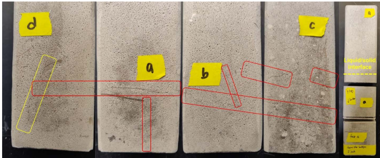
Figure 63. Four long faces of a geopolymer bar sample with 3% FABUTIT 748 addition after 20 cycles of thermal cycling immersion test
