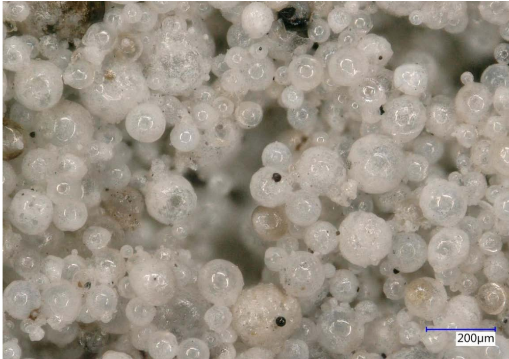
Figure 6. Optical microscope image of CenoStar ES500 cenospheres with the hollow sphere morphology
