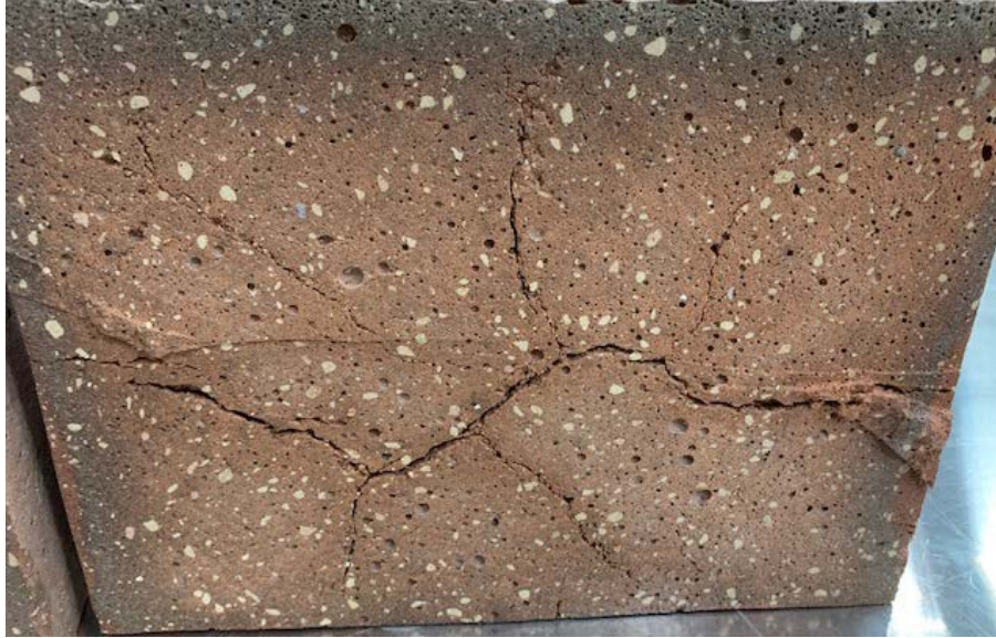
Figure 73. Interior cracks of the 50-lb geopolymer sample after 1,050°C firing
