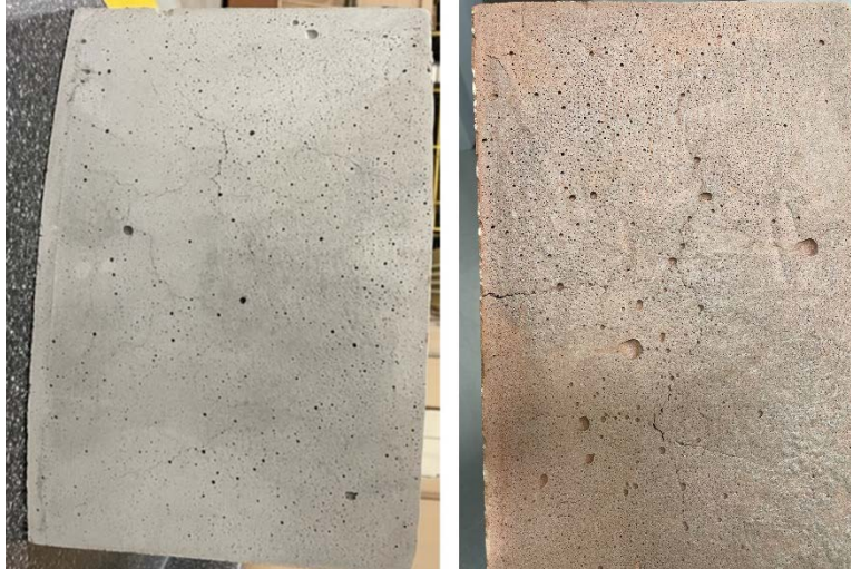
Figure 70. Comparison of one side face of a geopolymer brick before (left) and after (right) firing at 1,050°C
