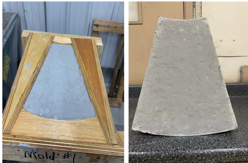
Figure 68. Pictures showing the geopolymer insulation after casting inside a mold (left) and after 7 days of curing at 60°C (right)
