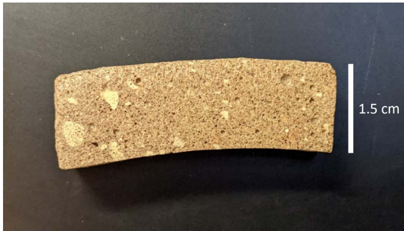
Figure 49. Geopolymer finger sample (1.5 cm × 1.5 cm × 5 cm) showing a significant dimension distortion after 1,200°C heat treatment for 5 hours
