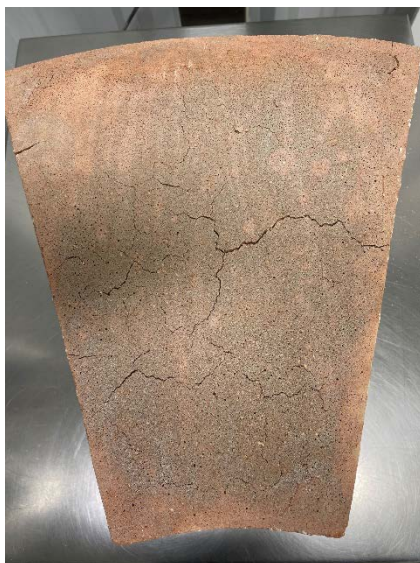
Figure 72. Bottom face of a geopolymer brick after firing at 1,050°C
