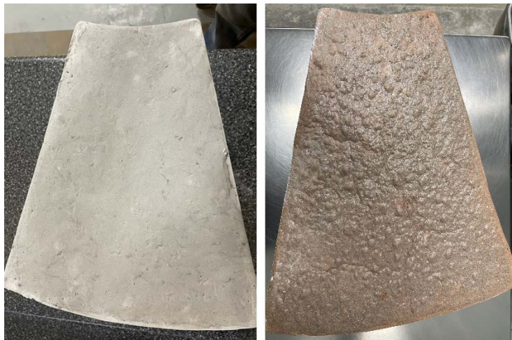
Figure 71. Comparison of the top face of a geopolymer brick before (left) and after (right) firing at 1,050°C
