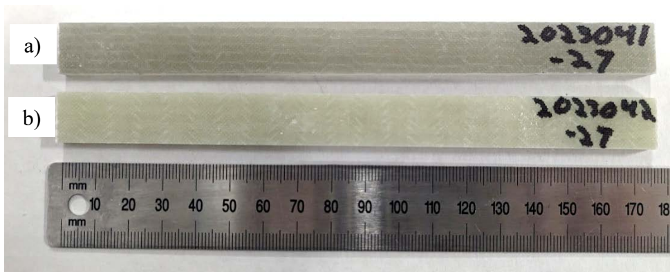
Figure 2. a) Vinyl ester composite coupon. b) Thermoplastic composite coupon.
