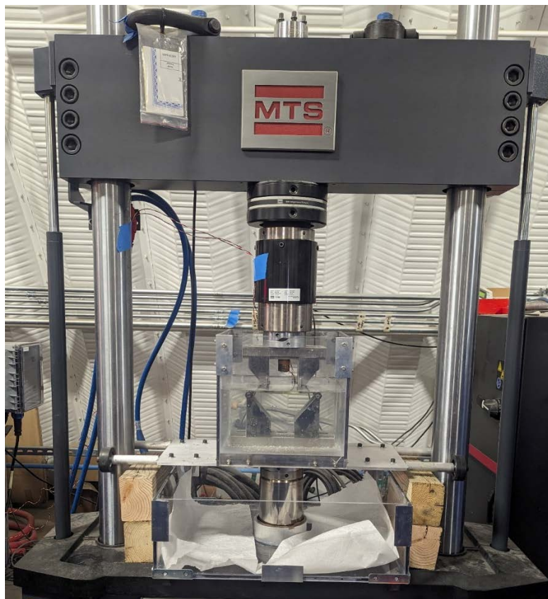
Figure 5. Photo of the as-built and installed load frame assembly in the 250 kN load frame.
