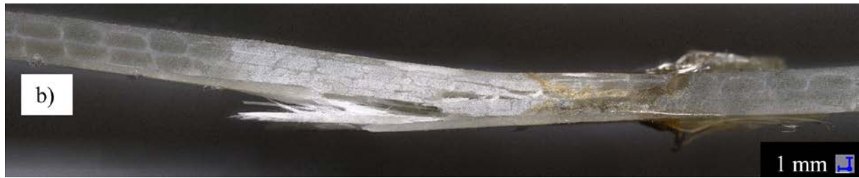
Figure 10. Microscope images at 3.7x magnification of two vinyl ester specimens that were a) dry fatigue-tested and failed at 17,418 cycles and b) fatigue-tested while submerged and failed at 13,125 cycles.
