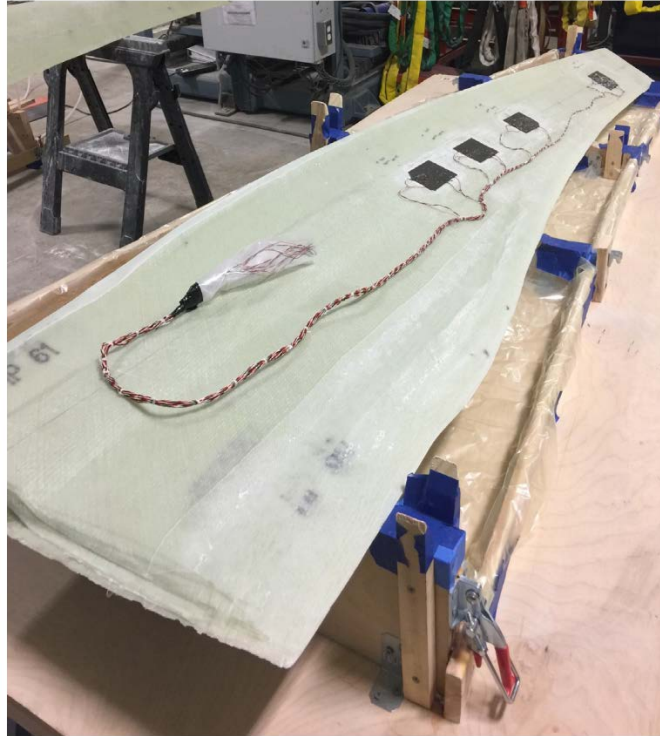
Figure 2. Fiberglass-reinforced Elium high-pressure skin with strain gauges bonded (photo by Robynne Murray).
