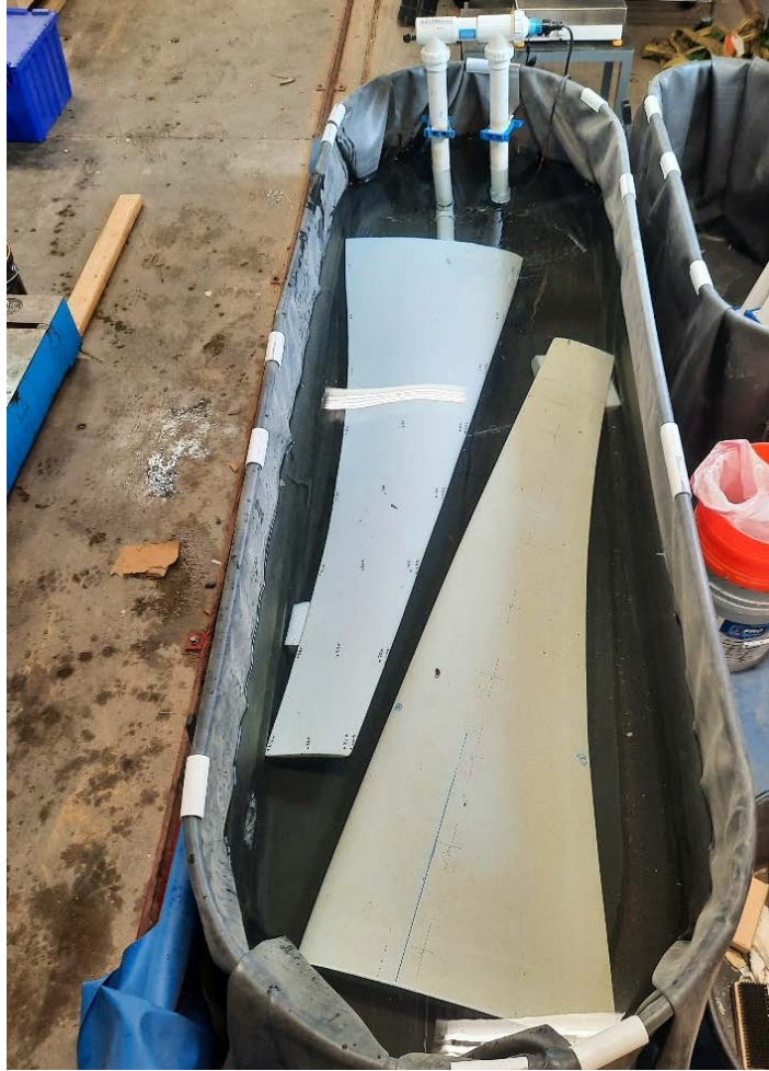
Figure 6. Fiberglass/epoxy and fiberglass/Elium blades being environmentally conditioned at ambient temperatures in a water tank.
