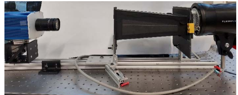
Figure 3. Bench-top transmission setup with pulsed flashlight with much less exposure time (<< 1 s)
