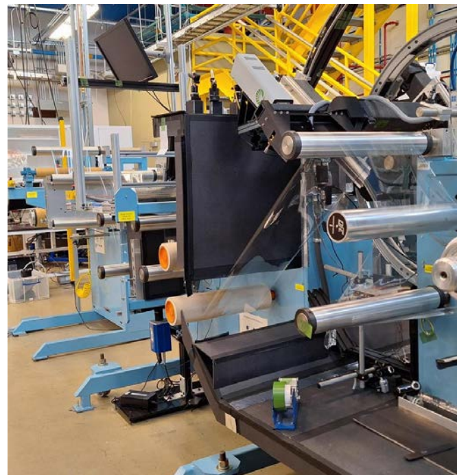
Figure 8. Transparent membrane thickness mapping through reflectance hyperspectral imaging while running the roll-to-roll system
