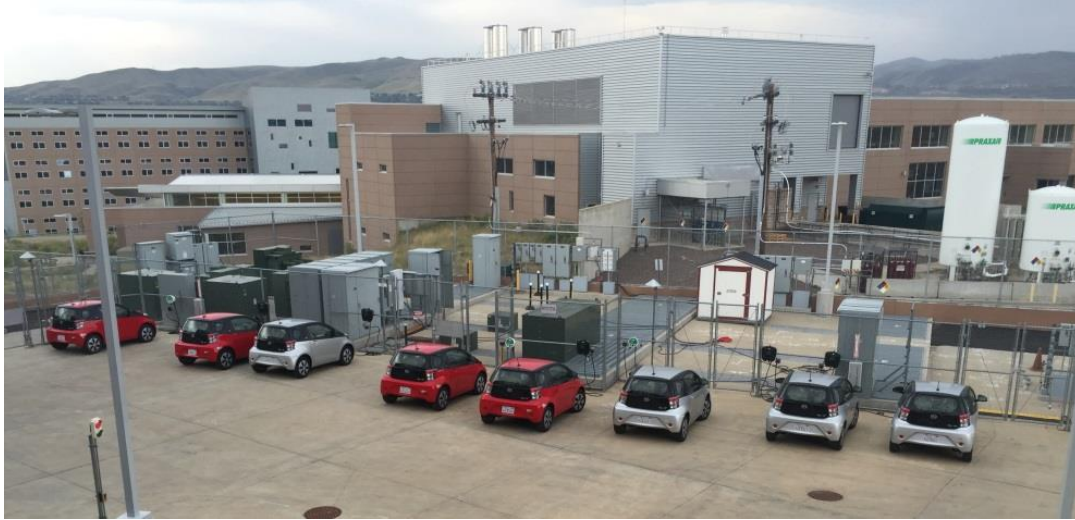
Figure 13: Prototype Toyota Scion iQ PEVs charging from the grid emulator
