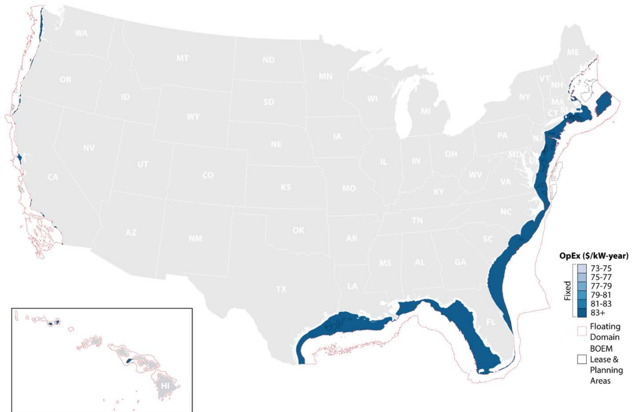
Figure 12. Fixed-bottom mid OpEx values [$/kW-yr] for the baseline year of 2025 in 2022 USD.
