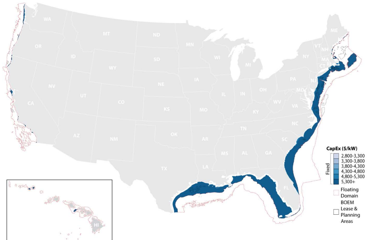
Figure 11. Fixed-bottom mid CapEx values [$/kW] for the baseline year of 2025 in 2022 USD.
