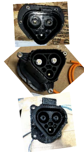
3x (Rema, T.E., Amphenol) 1800A MCS inlets on metal box w/ EVCC and bus bars (3000A)
