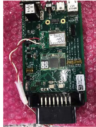
Modified ANL SpEC (CCS) module
