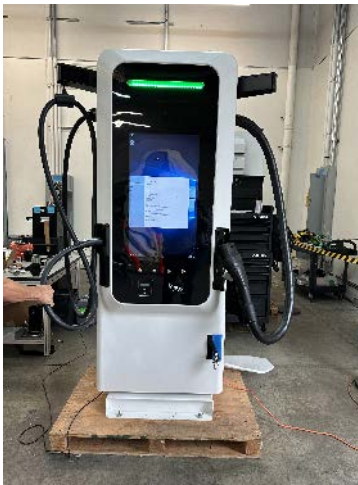
Dispenser with 3x MCS cables (~800A each); SECC controller inside
