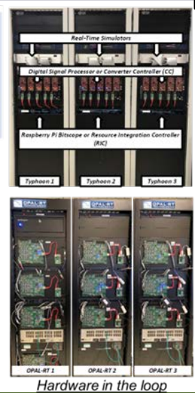
ORNL RT-simulation system for RT evaluation of control solutions and advanced technology prototypes
