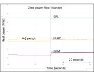
Successful planned islanding with GFM inverter HIL controlled through microgrid controller CHIL. GFL inverter is dispatched at rated power, leaving maximum capacity for GFM inverter to respond to net load steps. UCAP is activated because frequency dropped below 59.7 Hz.
