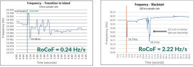
Successful island and blackstart with grid-forming inverter controlled through microgrid controller, arresting rate of change of frequency (RoCoF) and maintaining frequency within 59.7 – 60.3Hz.
