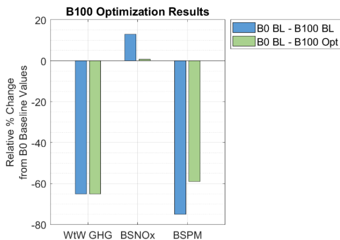
Figure 13. Comparison of results for the original engine calibration with the B100 calibration for greenhouse gas emissions, NO x , and particulate matter.
