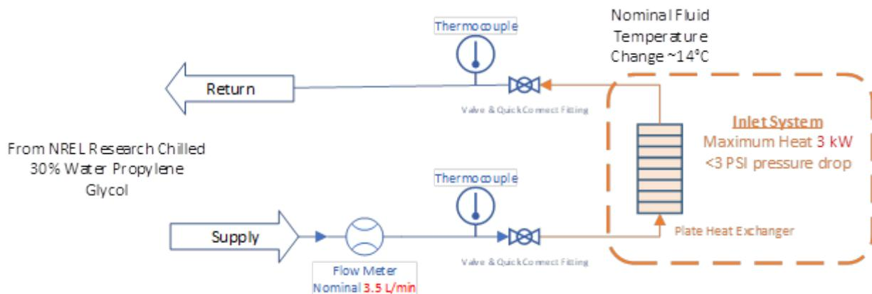
**Figure 5. Simplified MCS 3000A Inlet Cooling System Diagram**
