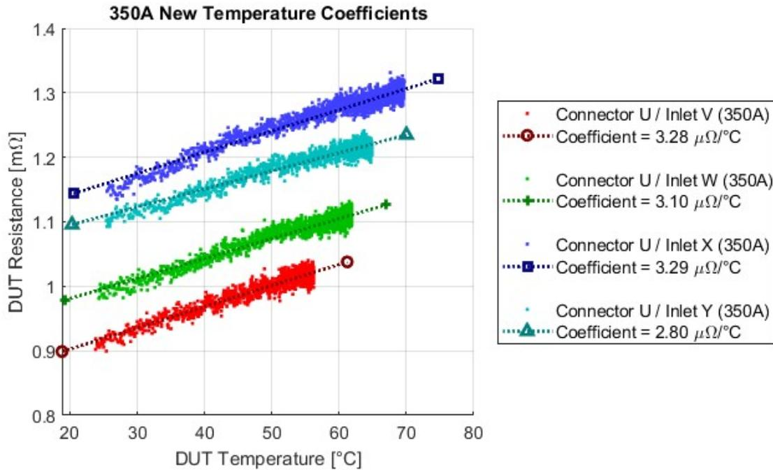
**Figure 10. MCS 350A New Connector/Inlet Temperature Coefficients of Resistance**
