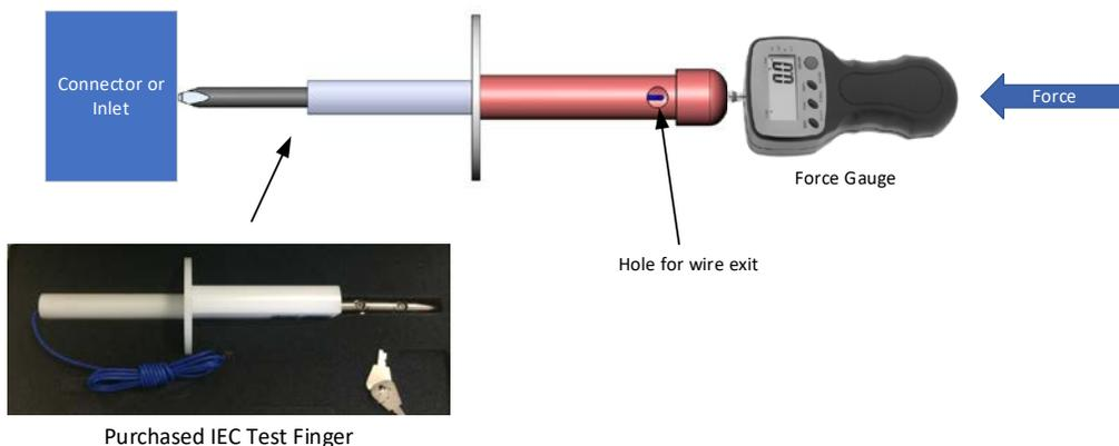
Figure 24: IEC Touch-Safety Finger Setup
