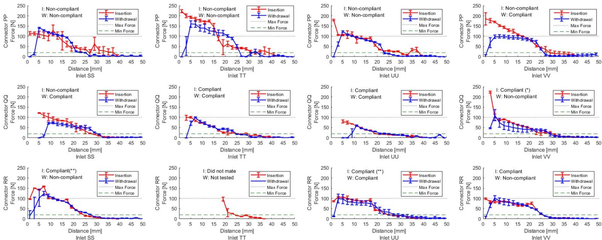
**Figure 22: Insertion and Withdrawal Force vs. Distance**
