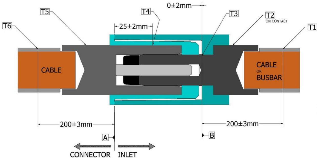
**Figure 1. Thermocouple locations at the connector/inlet interface**
