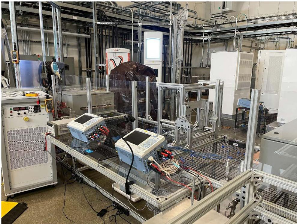
**Figure 9. MCS Thermal Interoperability Evaluation Bench Setup with Safety Guards.**
