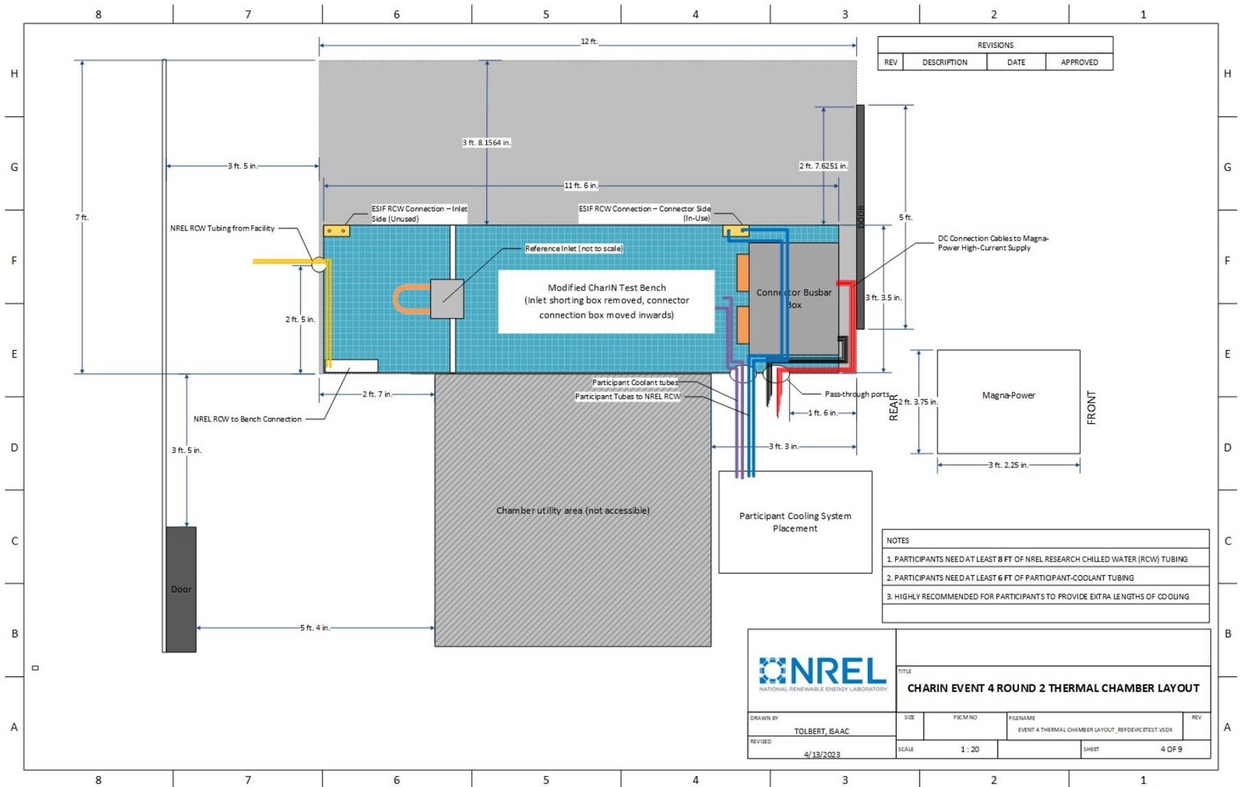
Figure 18: Schematic of thermal chamber and test bench setup, showing cooling and electrical connections
