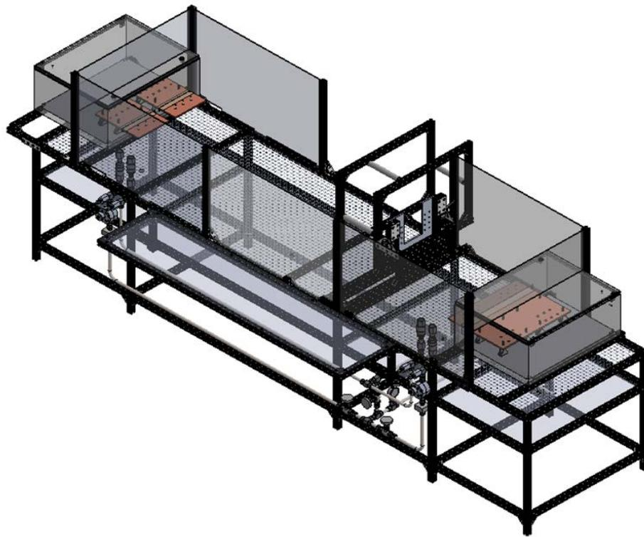
**Figure 8. MCS Thermal Interoperability Evaluation Bench Safety Guards.**
