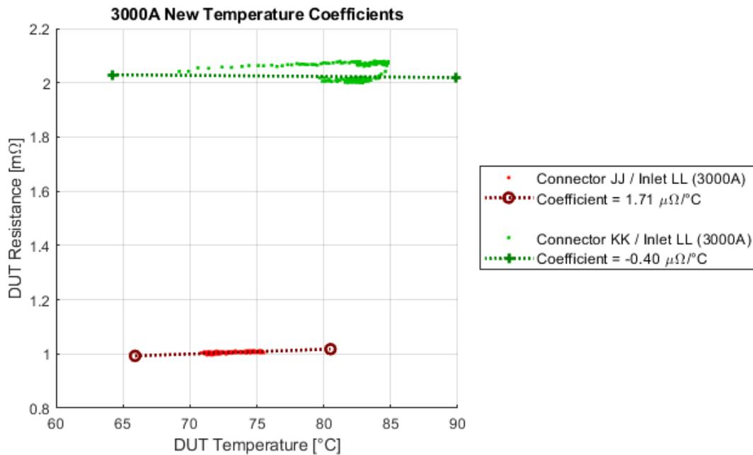
**Figure 13. MCS 3000A New Connector/Inlet Temperature Coefficients of Resistance**
