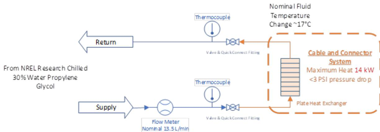
**Figure 4. Simplified MCS 1000A-3000A Connector Cooling System Diagram**
