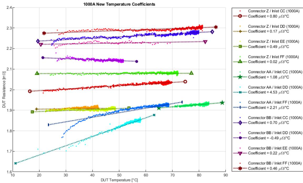
**Figure 11. MCS 1000A New Connector/Inlet Temperature Coefficients of Resistance**
