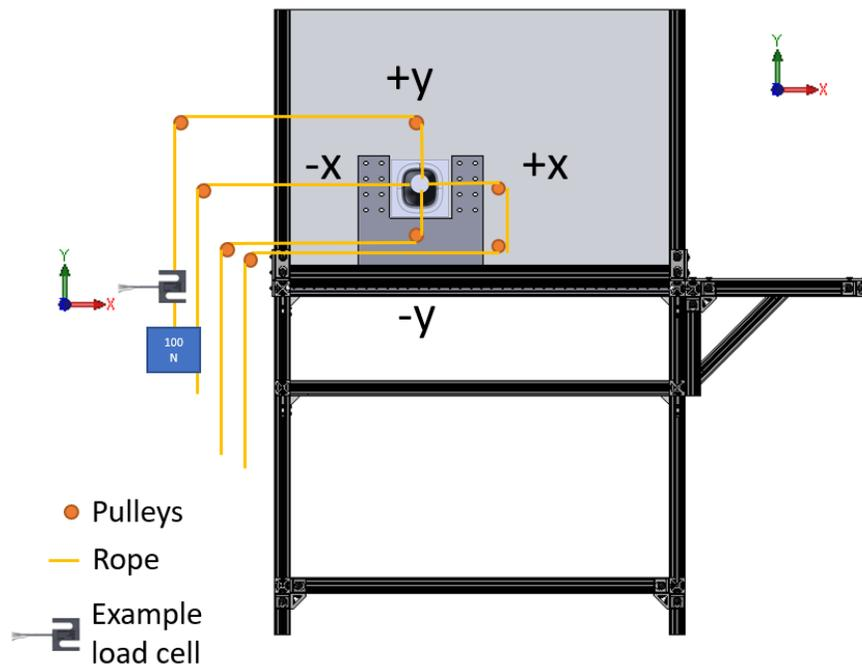
**Figure 15. Layout of misalignment test setup with 100N load, facing towards the inlet from the connector end of bench**
