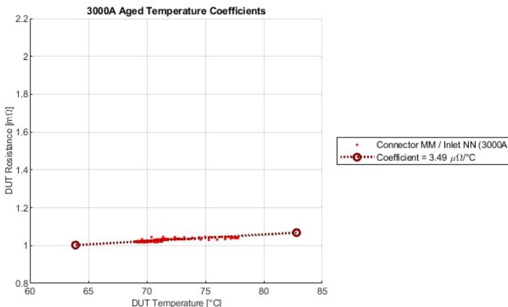
**Figure 14. MCS 3000A Aged Connector/Inlet Temperature Coefficient of Resistance**
