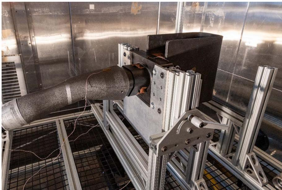
**Figure 17: 3000A Reference Device with Connector Attached**
