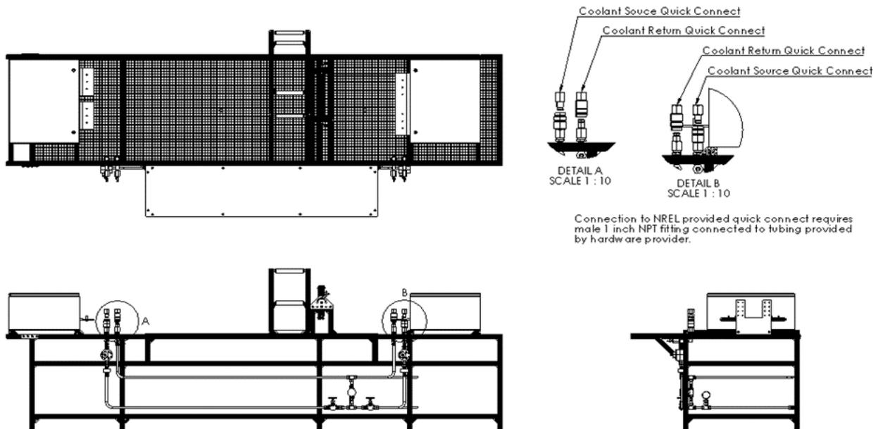
Figure 3. CharIN Thermal Interoperability Evaluation Bench and Cooling System Dimensioned Plan and Elevation Views
