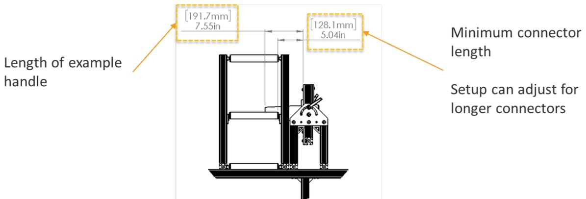
**Figure 7. Side view of force alignment frame.**
