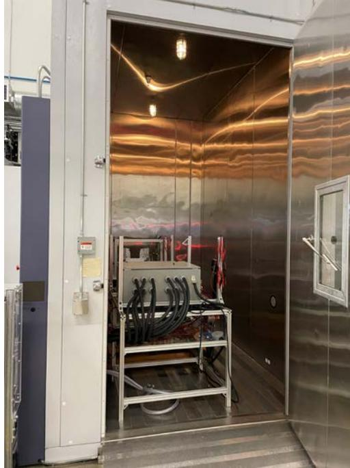
**Figure 19: Exterior view of thermal chamber and evaluation bench**
