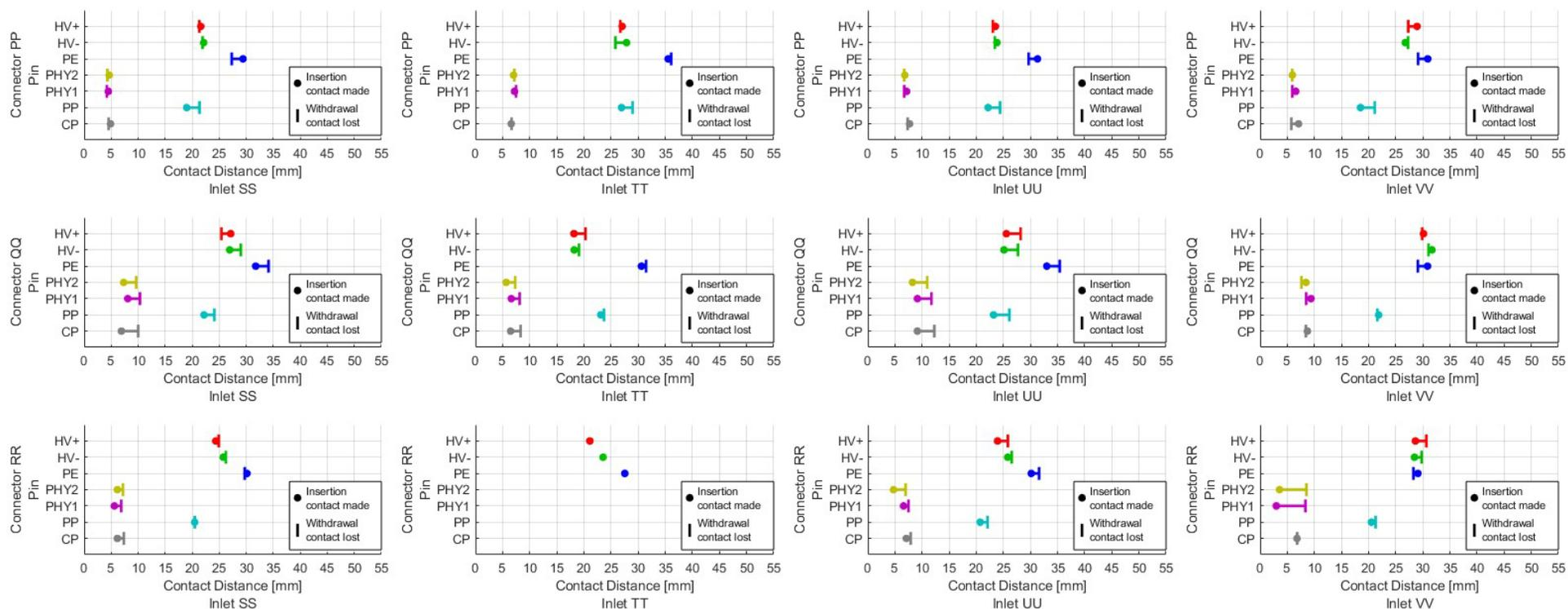
**Figure 23: Insertion and Withdrawal Pin Contact Sequence**
