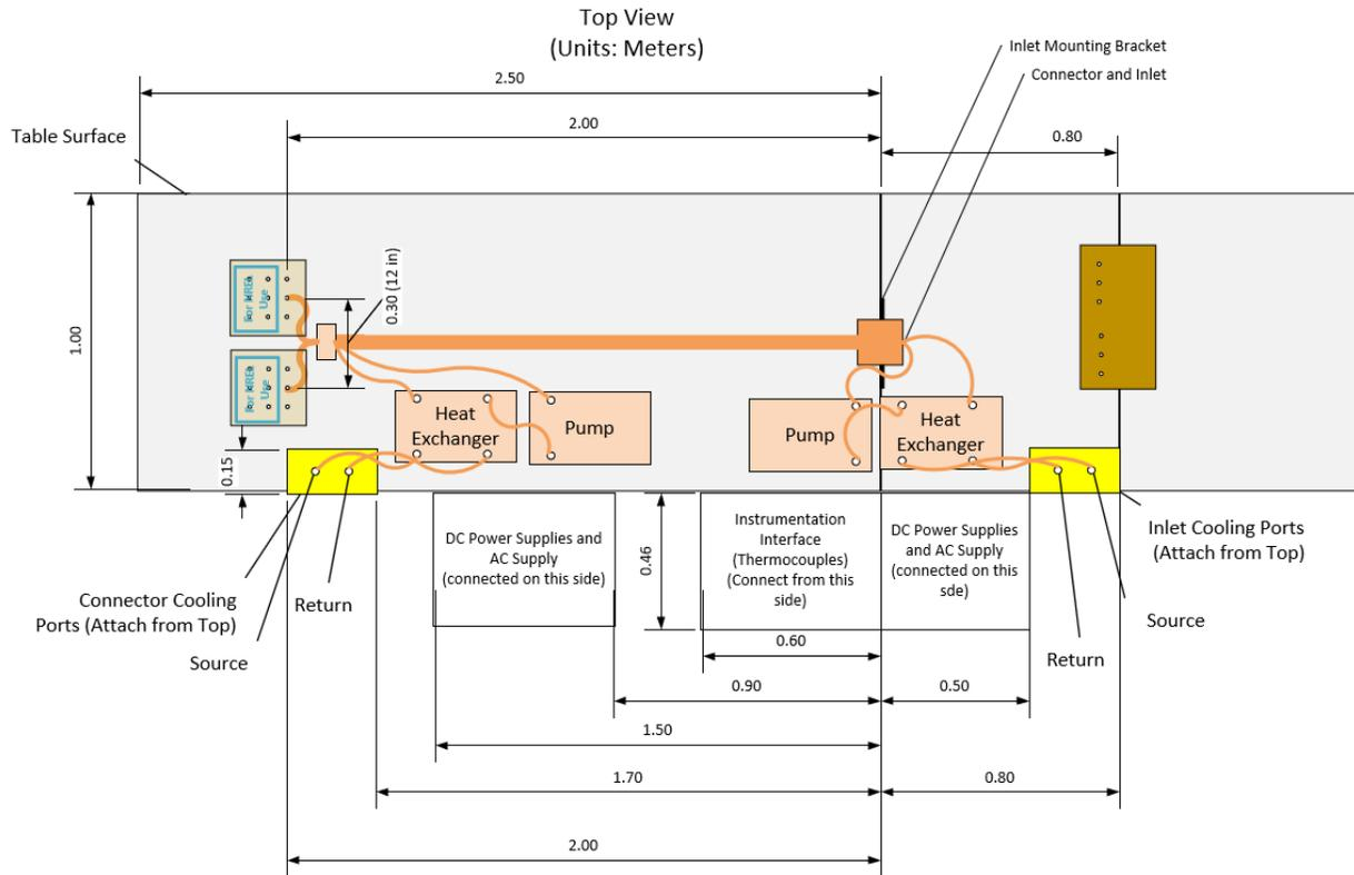
Figure 2. CharIN Thermal Interoperability Evaluation Bench Layout
