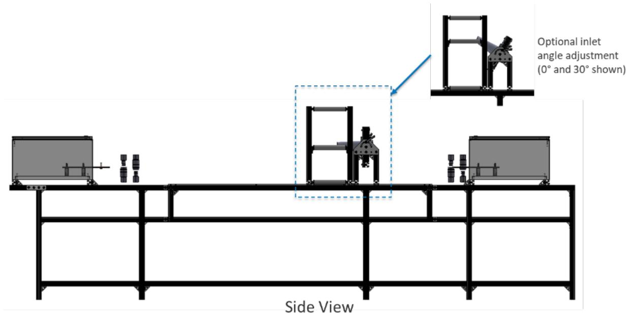
**Figure 6. Force application frame with inlet attachment frame mounted on test bench.**
