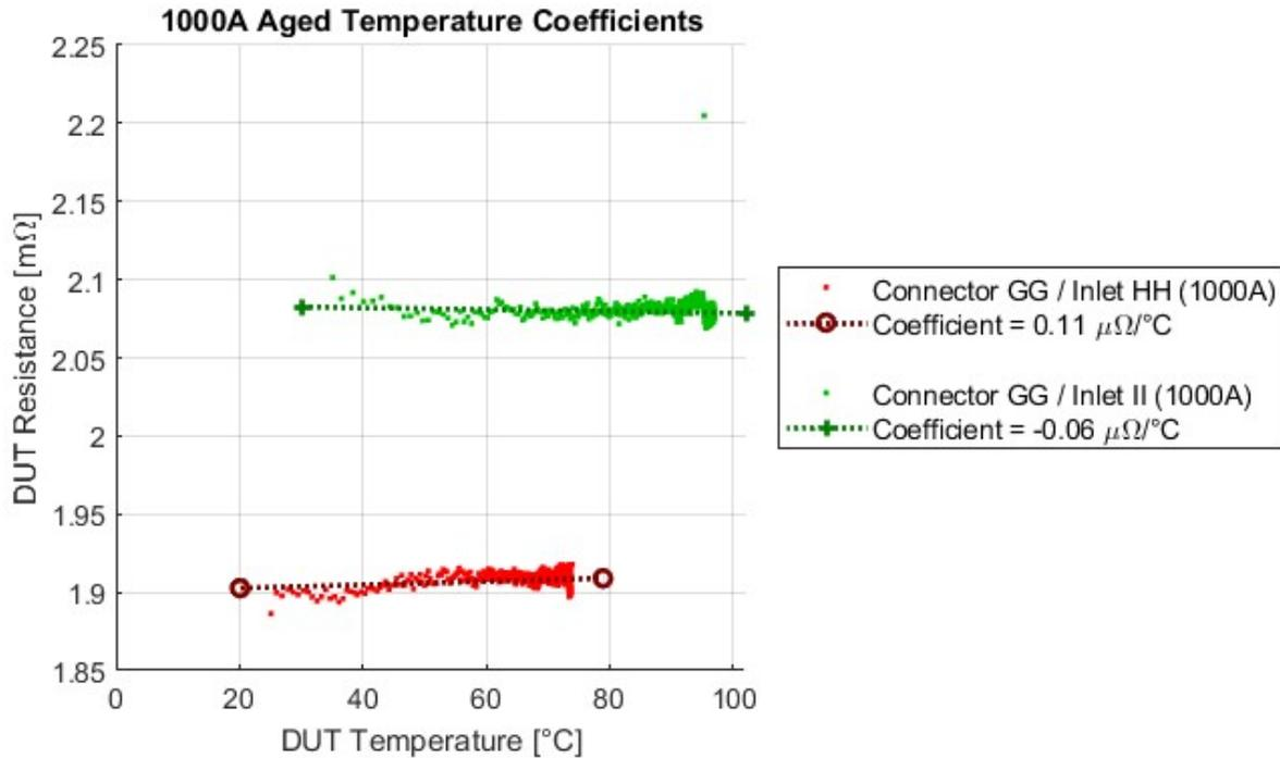
**Figure 12. MCS 1000A Aged Connector/Inlet Temperature Coefficients of Resistance**
