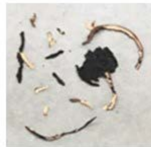
Si@pitch with PI binder 4 mAh/cm 2
