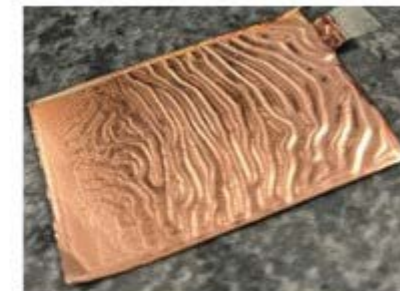
SiO x with PI binder 4.5 mAh/cm 2
