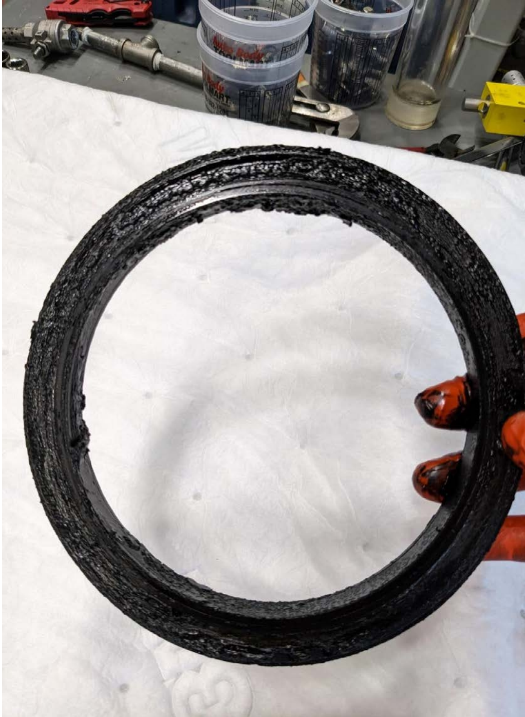
Figure A-5. Wear surface of the front graphite antifriction ring with accumulation of graphite/BF residue. The visible surface interfaces with the bronze seal face ring.
