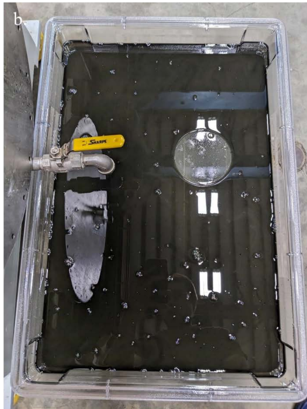
Figure 5. Images showing the fluid removed from the water tank: (a) side view; (b) top view. The BF floats on top of the water and is stained black from suspended graphite particles worn away from the antifriction rings.
