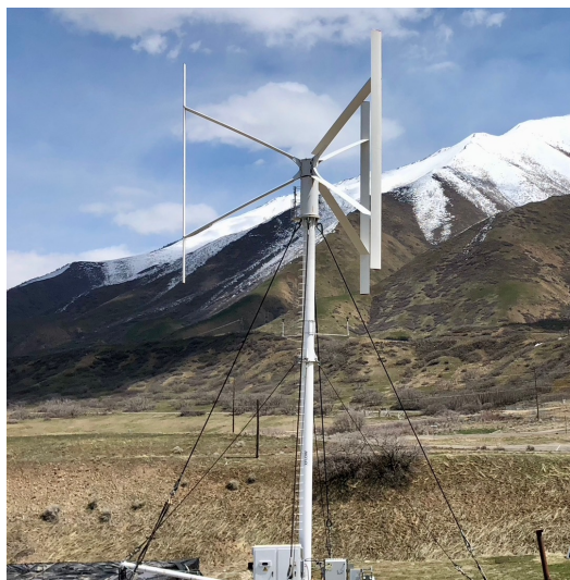
(a) XFlow Energy Co. 10-m turbine showing configuration and overall geometry.
