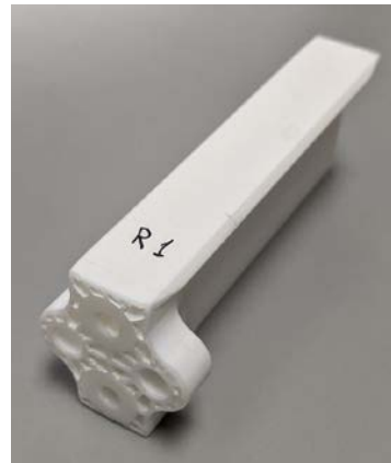
T-shape in-slot heat exchanger 3D-printed from Rigid 10K resin at NREL. Photo by Bidzina Kekelia, NREL
