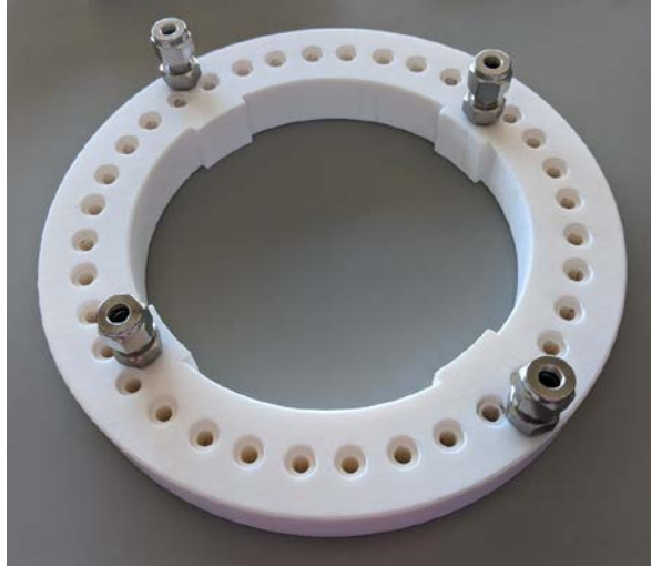
Coolant distribution manifold with inlet-outlet fittings (back) and attached T-shape in-slot heat exchangers (front). Photos by Bidzina Kekelia, NREL
