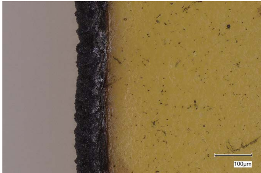
HAZ of 9.3- \mu\text{m} commercial CO 2 laser
