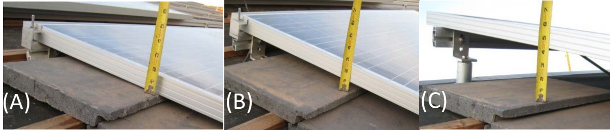
Standoff images for distances of (A) flush mount (B) 2.5 cm, and (C) 10 cm.
