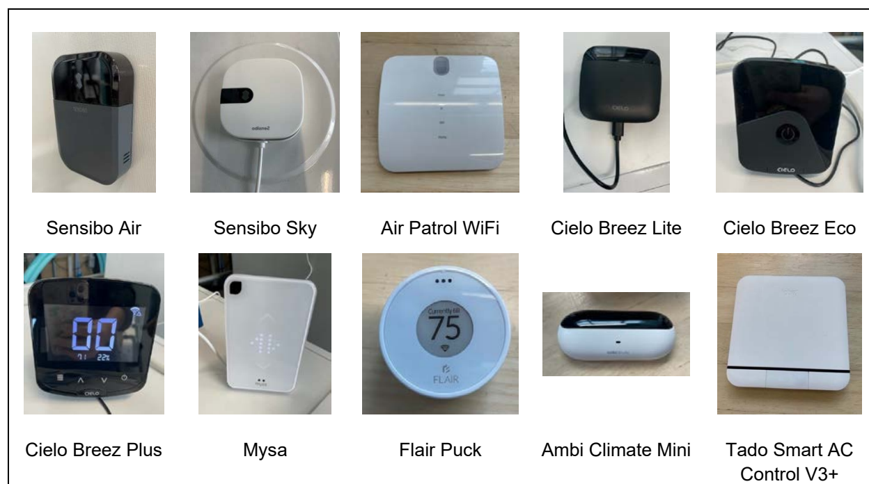
Figure 2. Third-party connected thermostats for room ACs and MSHPs
