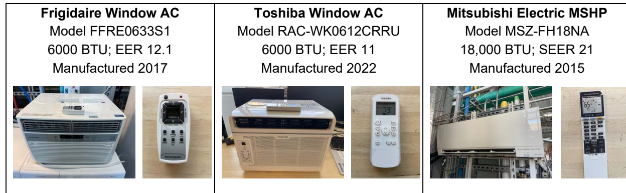
Figure 1. HVAC units and their remote controls used for thermostat testing
