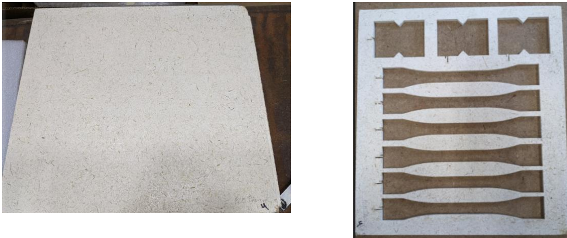
Figure 1 – As-delivered geopolymer panel (left), and geopolymer panel after coupons were cut via water jet (right)
