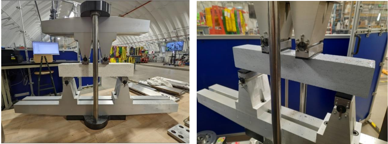
Figure 5 – Geopolymer beam specimens in a long beam test fixture
