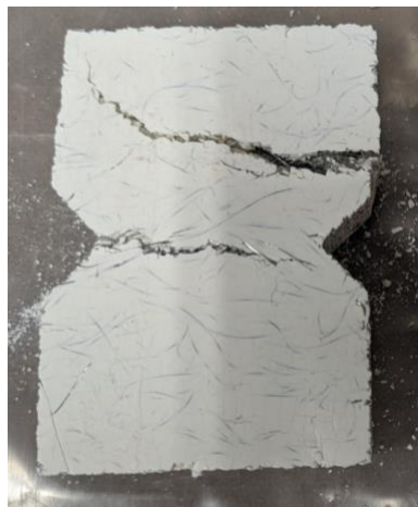
Figure 7 – Geopolymer shear coupon, post-failure
