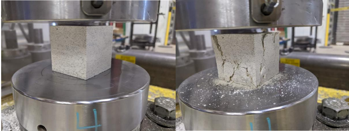
Figure 8 – Geopolymer compression cube before loading (left) and post-failure (right)
