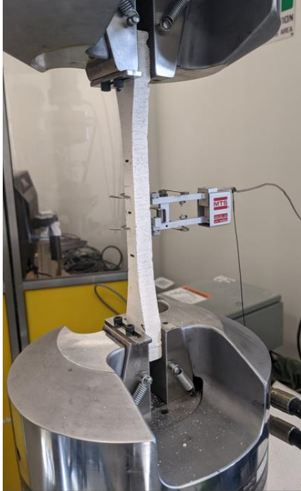
Figure 6 – Geopolymer tensile specimen in the 100 kN load frame (left), post-failure tensile specimens (right)
