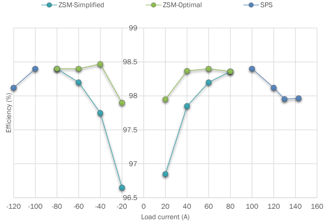
Efficiency results at 900 V in Buck/Boost mode
