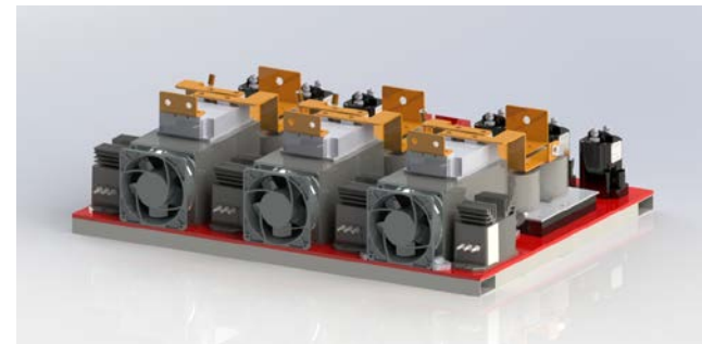
2 kV class 175/350 kW DC/DC charger CAD
