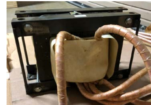
1 kV Class 200 A, 20 kHz Nanocrystalline Transformer
