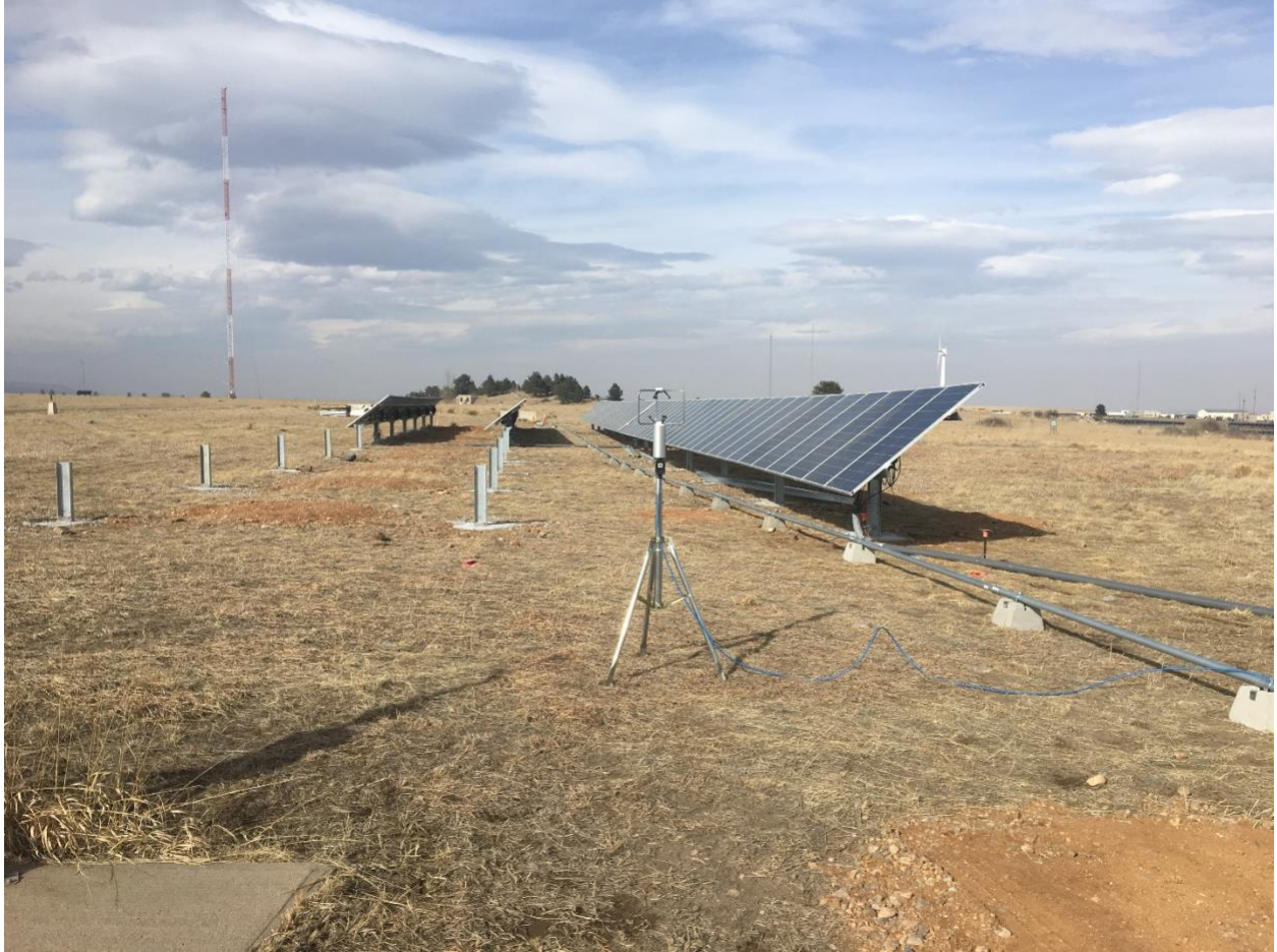
Figure 4. Sunfolding test array with sonic anemometer in the foreground (Photo: Jerry Hur, NREL))
