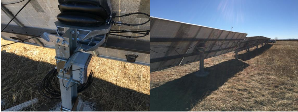
Figure 12. R&D prototype of locked actuator for extremely high wind applications. The concept showed some promise but needed extensive re-design due to results at HWTS.
