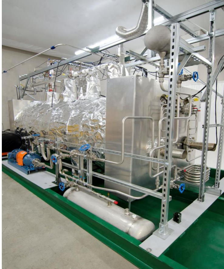
Figure 1. Element16's 350 kWh sulfur TES prototype
