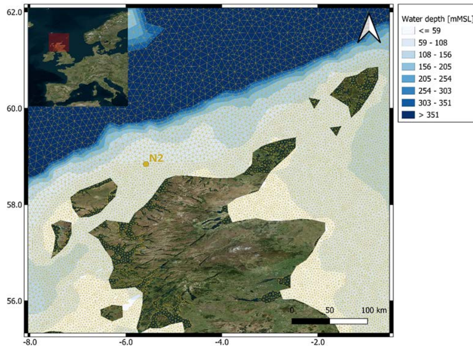
Figure 12. Analysis location (N2) used to represent the Havbredey project with the mesh and bathymetry of DHI’s hydrodynamic UK and North Sea model.
