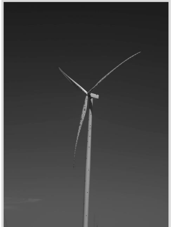
NREL researchers triggered faults on this wind turbine in Texas caused by structural loads, resulting in the tower deflection shown here. The markers on the tower and blades were used to measure these motions.
