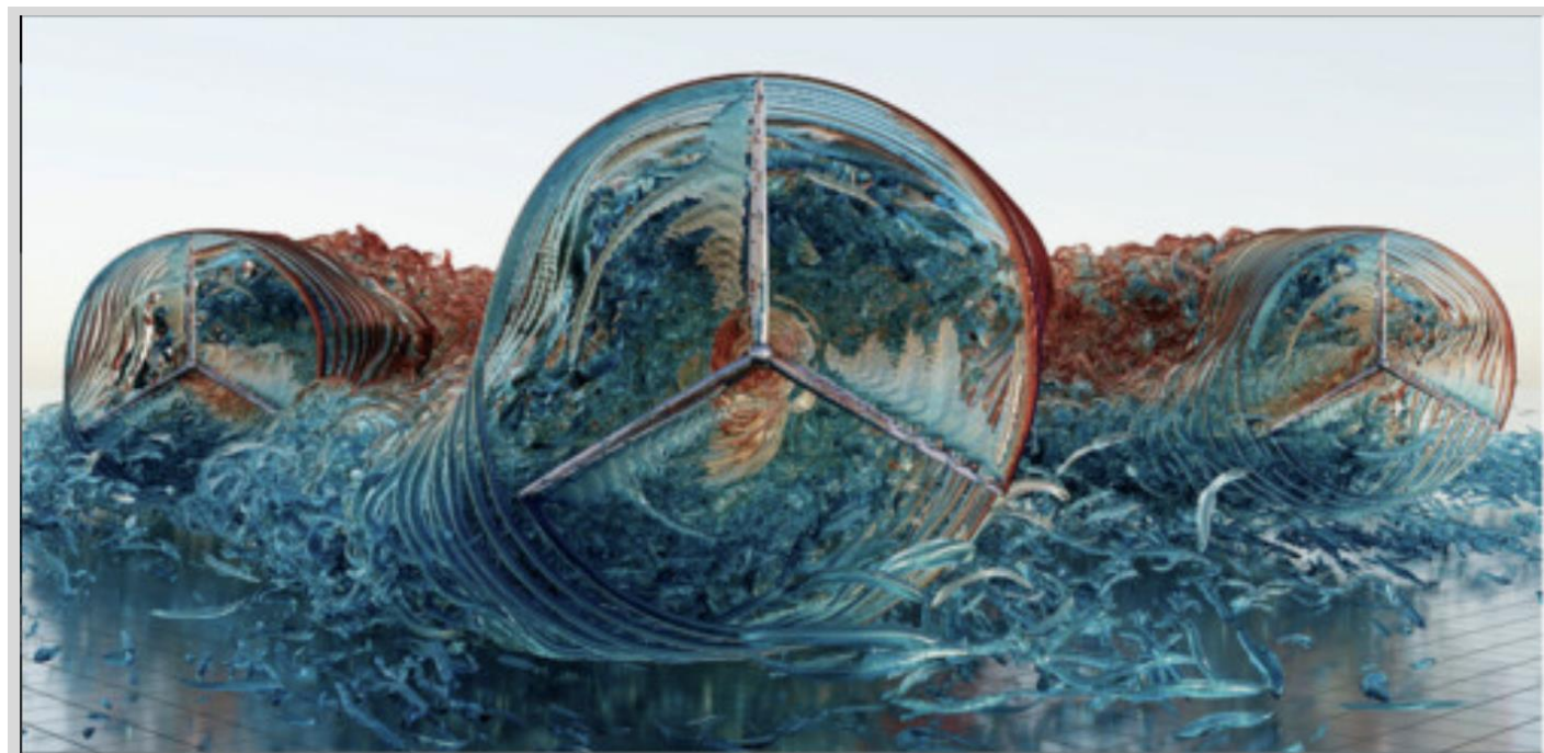
Researchers developed an ExaWind simulation of four NREL 5-MW wind turbines in a turbulent atmospheric flow, illustrated here. Graphic by Nicholas Brunhart-Lupo, NREL
