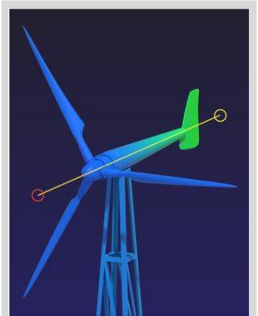
NREL's OpenFAST wind turbine simulation tool now includes code for modeling tail-vane-controlled, passive-yaw wind turbines, like the one pictured here. Graphic by Besiki Kazaishvili, NREL
