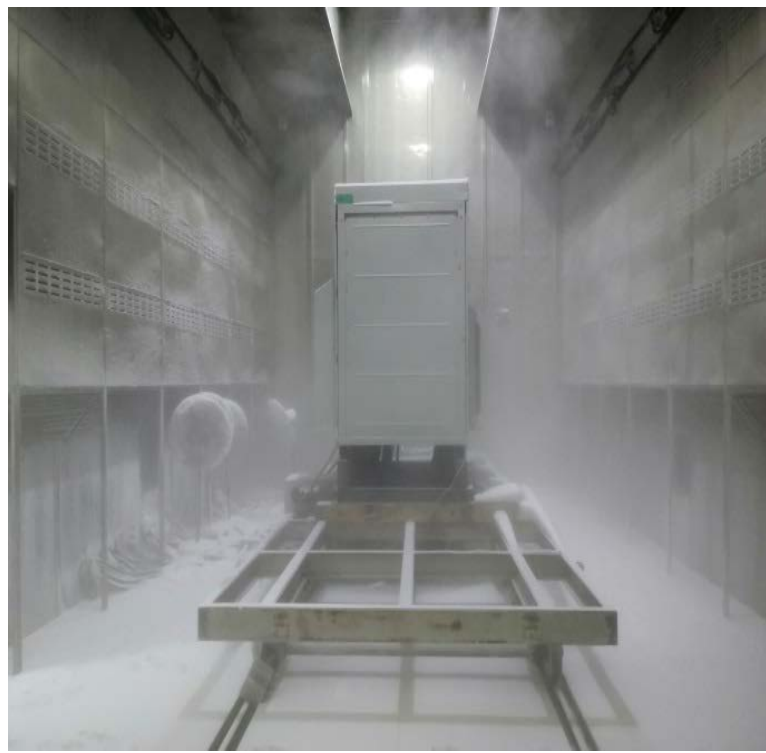
Snowfall test: snowfall thickness 10cm
