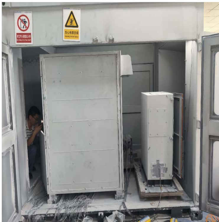
Sandstorm test: Sandstorm 32m/s, sand dust 75-135um
