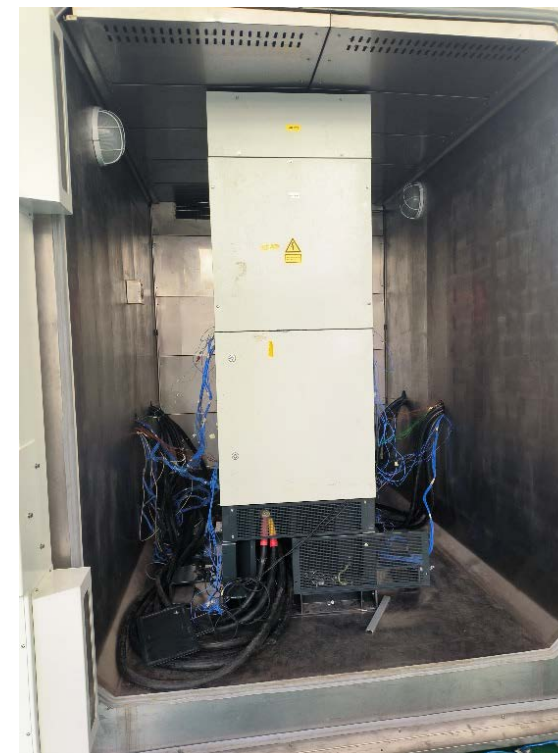
High altitude and low pressure testing
