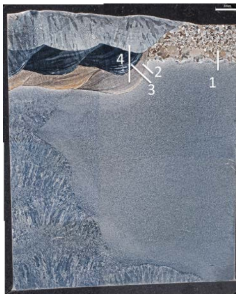
Figure 43. EDS line scan locations in the cross section of butt-welded 91 steel backer with Ni201 clad
