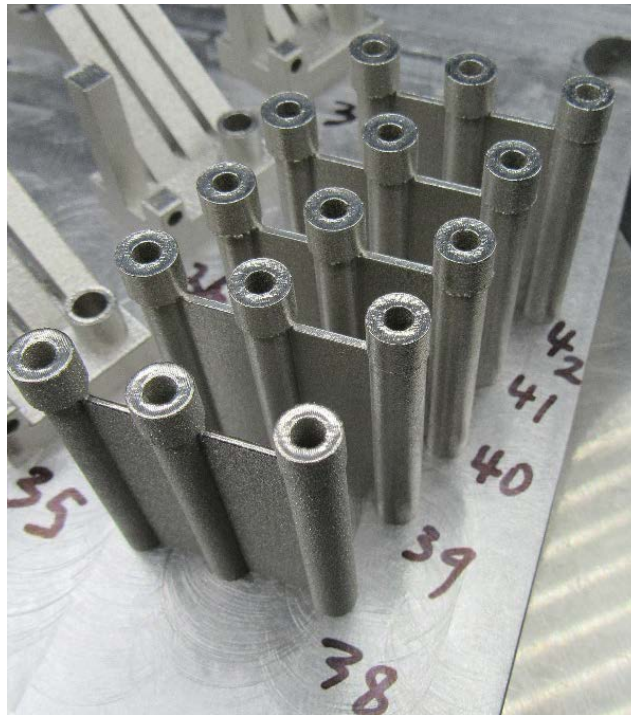
Figure 104. In740h pressure tubes with contours. No set of tubes leaked after being subjected to 4 bars of air pressure.
