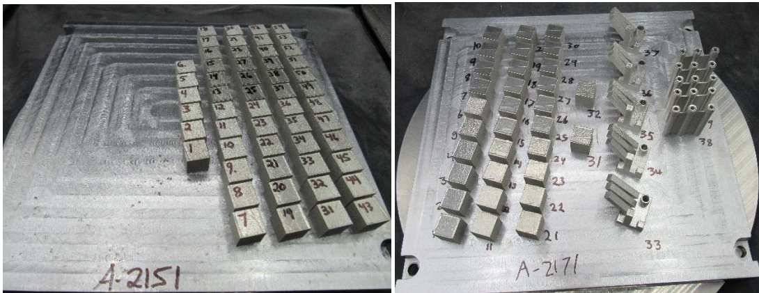
Figure 97. The In740h development builds showing the coupon designs utilized to fulfill the required criteria for Build 1 (left) and Build 2 (right)
