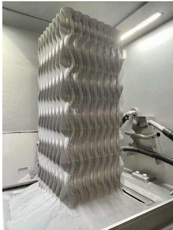
Figure 249. Sintavia large AM HX for marine use.
