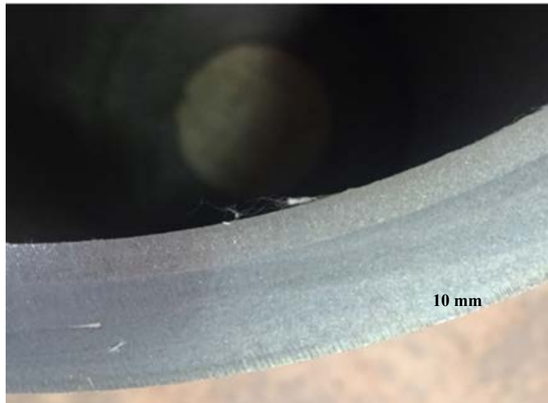
Figure 6. A ~4-mm-thick SS316 cladder on a carbon steel backing pipe (27 mm OD, 12 mm thick, 500 mm long) using CS/CR. Courtesy of AMS
