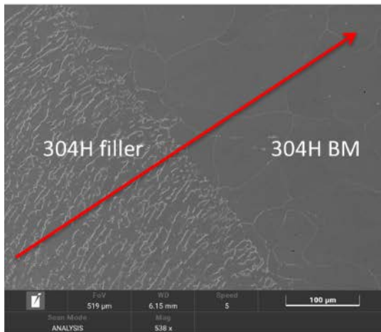
Figure 39. EDS scan (line 4 in Figure 27) from 304H filler to 304H substrate
