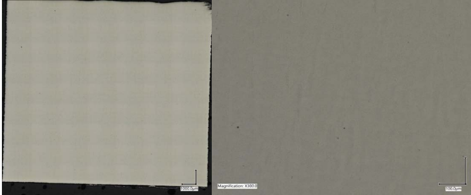
Figure 96. Development build A for H282 cube 15. 100X image stitch of the whole cube (left) and 300X closeup (right)
