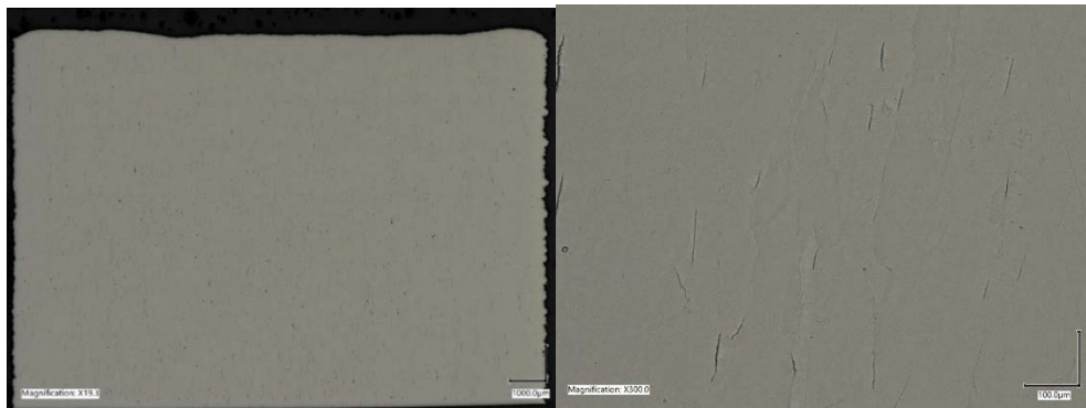
Figure 95. Development build B, alloy 230, cube 10 (microcracking present.) Columnar grain growth was observed with cracking around the grain boundaries. The energy density used was 119 J/mm 3 . 100X image stitch of the whole cube (left) and 300X closeup (right)
