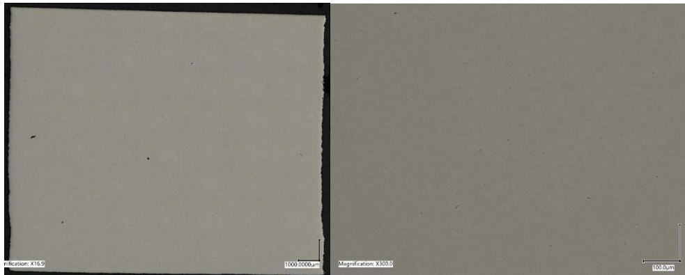
Figure 94. Development build A, alloy 230, cube 17. The cube used an energy density of 119 J/mm 3 . 100X image stitch of the whole cube (left) and 300X closeup (right)
