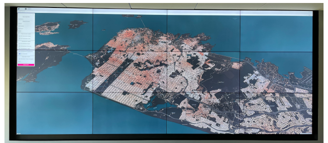
Figure 3: San Francisco SMART-DS model on the Insight Center 100 megapixel display wall. Assets are styled from time-series values with a diverging color-scale based on nominal per-unit voltage (white) and +/-5%, with red as higher and blue as lower voltages.
