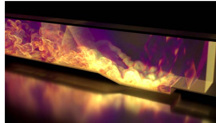
Supersonic cavity flame holder Sitaraman et al., Combustion and Flame, 2021
