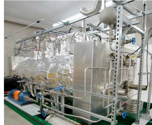
Element 16's 350KWh pilot sulfur TES prototype
