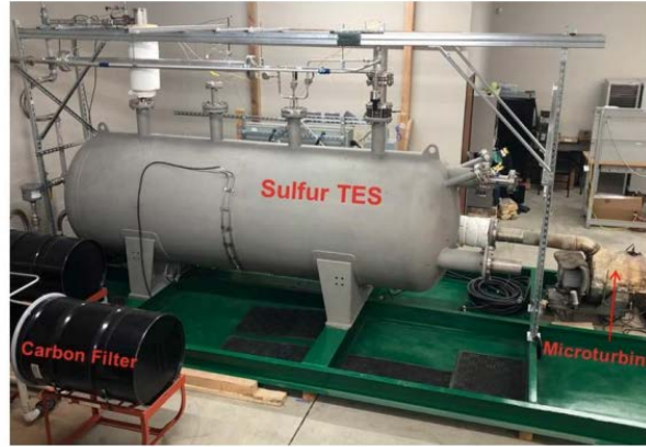
Element 16's 350KWh pilot sulfur TES prototype
