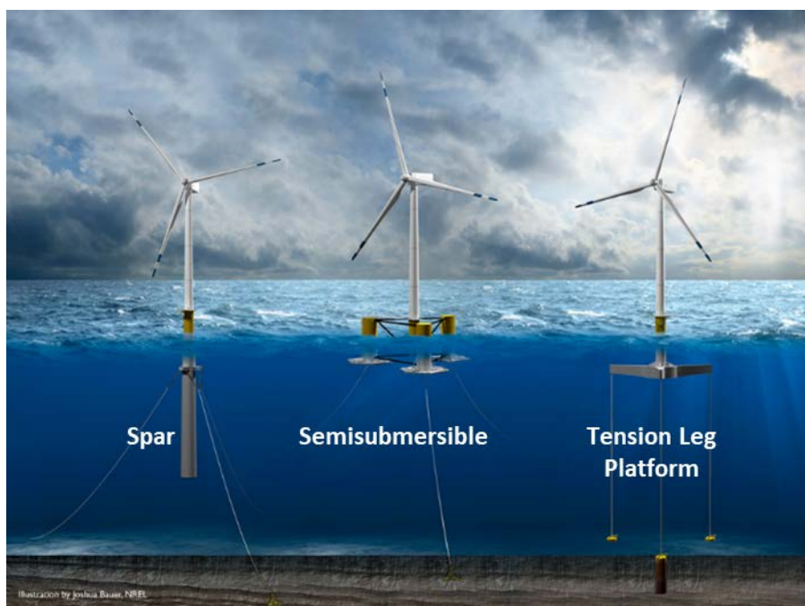
Figure 19. Substructure types for floating offshore wind systems including the spar buoy, semisubmersible, and tension-leg platform. Illustration by Josh Bauer, NREL
