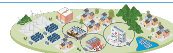
Scenario 1: Economic Rooftop solar and storage adoption based on financial savings and value of backup power to building owners and prioritized for critical services (circled) .
