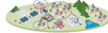
Scenario 3: Maximum Rooftop solar and storage is added to all suitable rooftops to meet critical loads.
