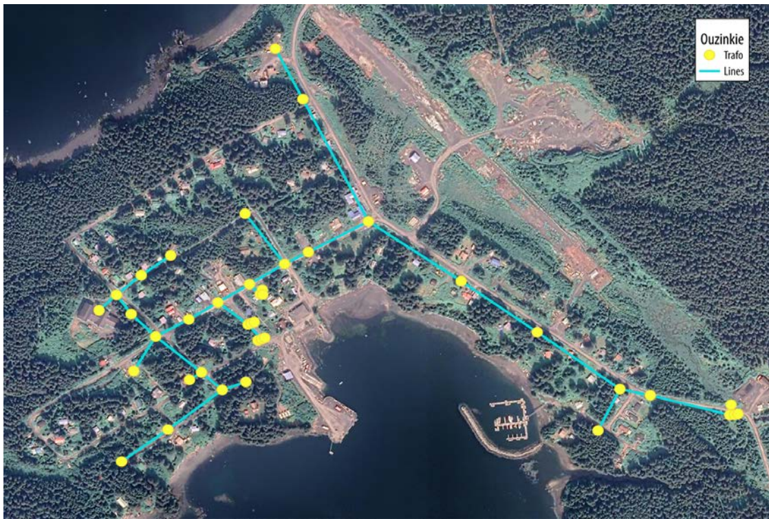
Figure 19. Ouzinkie electrical distribution system. Transformer locations are indicated by yellow dots. Image from Google Maps.
