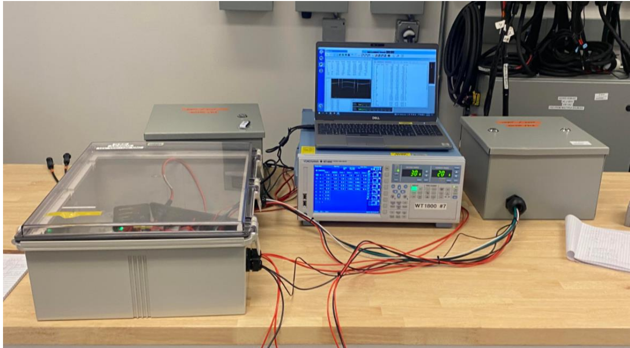
Figure 3. JuiceBox 3.0 unit under test. Visible are (left to right) input wiring box; power analyzer; unit under test; output wiring box; electronic load. Photo by Andy Walker
