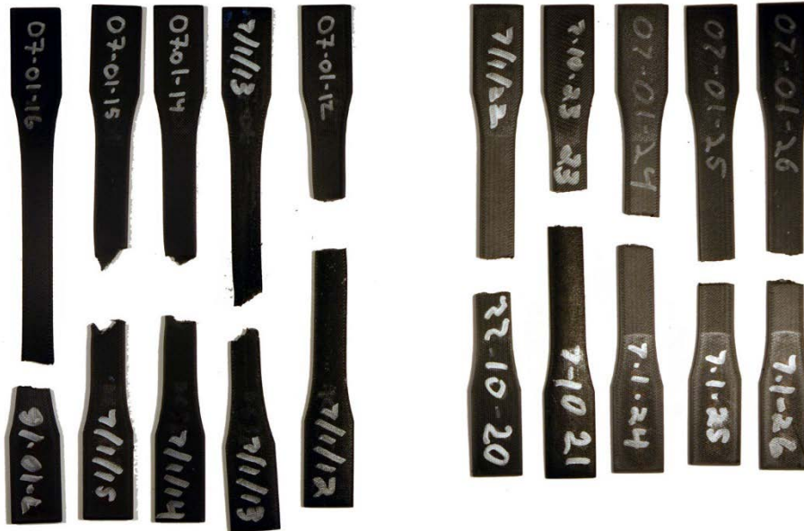
Figure A-5. Photo of ASTM D638 tensile-tested Onyx material series
