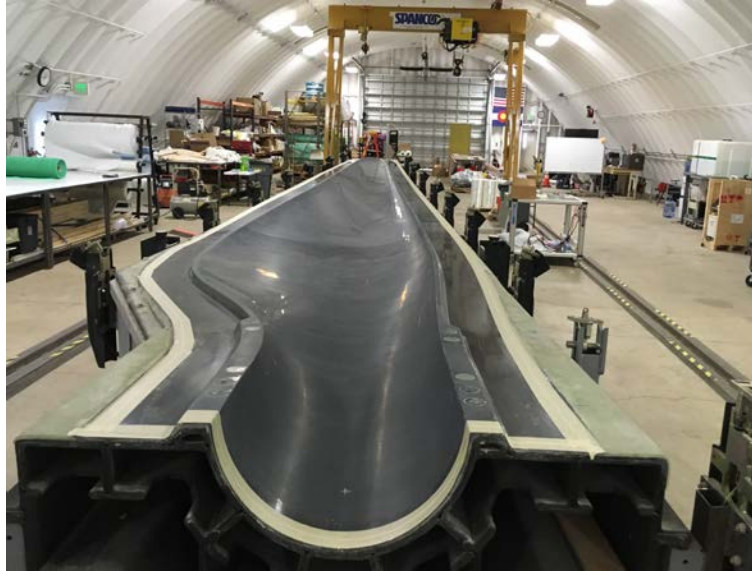
Figure 2. A 13-meter wind turbine blade mold that was 3D-printed with chopped carbon fiber/acrylonitrile butadiene styrene, manufactured by Oak Ridge National Laboratory and TPI Composites
