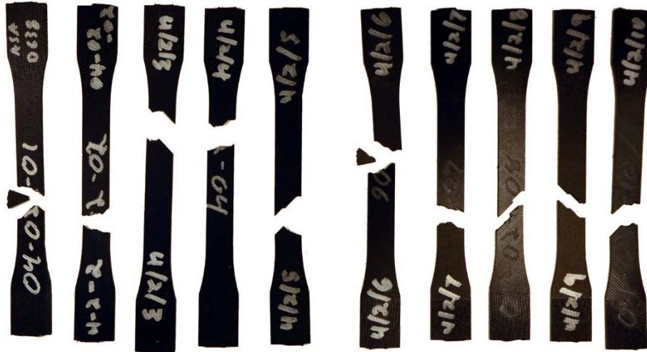
Figure A-3. Photo of ASTM D638 tensile failures in the ASA specimens
