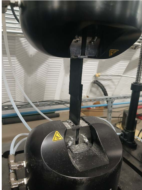
Figure 28. A 3D-printed polymer/strain gage adhesive lap shear specimen being tested in the load frame
