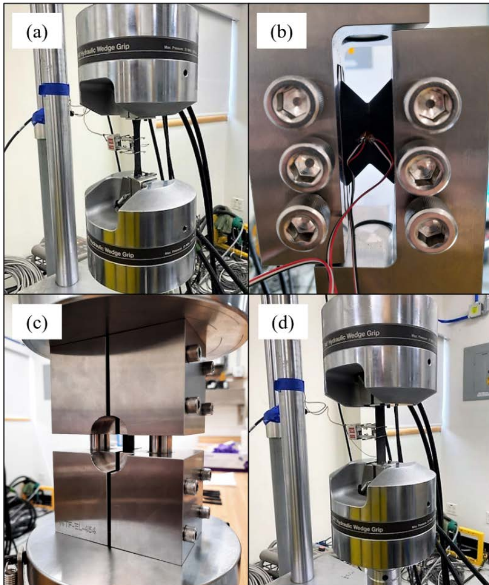
Figure 14. Examples of the test methods applied: (a) ASTM D638 tension, (b) ASTM D7078 shear, (c) ASTM D6641 compression, and (d) ASTM D3039 tension
