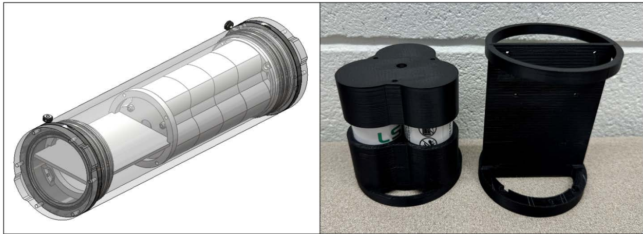
Figure 41. CAD drawing of the black box data acquisition system featuring 3D-printed electronics mounting and battery housing (left) and a photo of the 3D-printed components (right)
