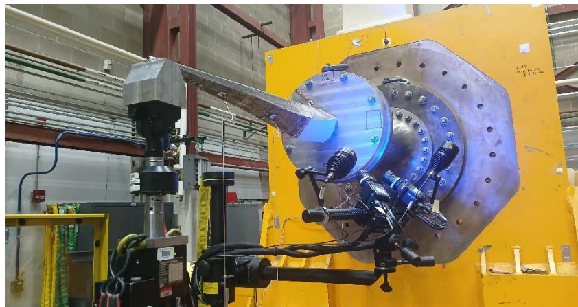
Figure 3. Structural validation of a 3D-printed tidal turbine blade spar manufactured using DED and 316L stainless steel
