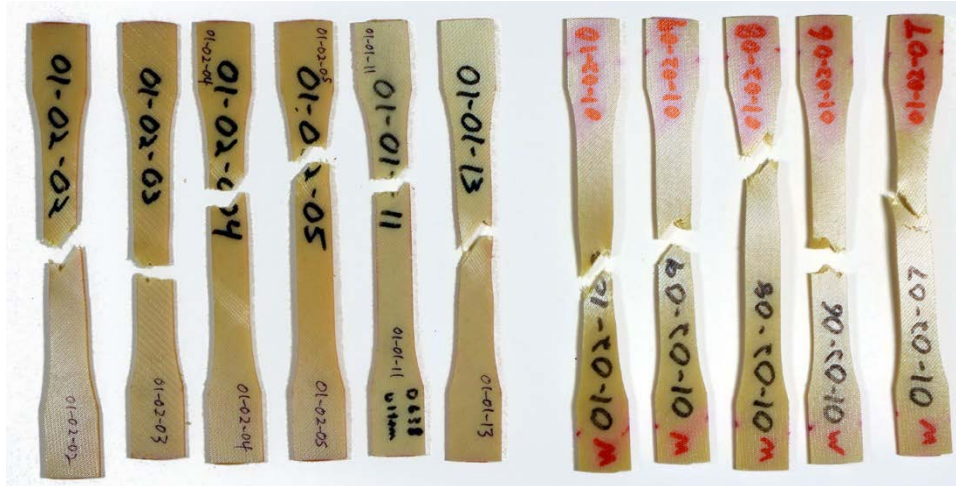
Figure A-1. Photo of ASTM D638 tensile-tested Ultem 9085 series
