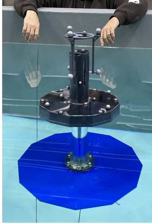
Figure 38. 3D-printed RM3 model being tested at NREL’s Sea Wave Environmental Laboratory
