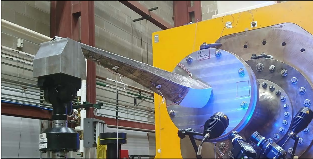
Figure 42. A photo of the 316L stainless steel turbine blade spar mounted to the structural test stand
