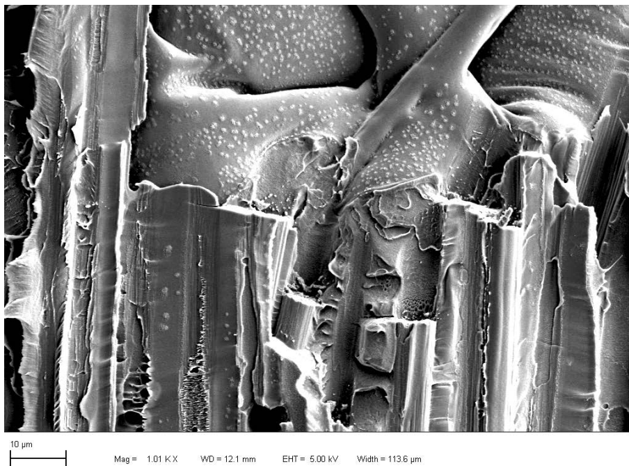
Figure A-14. Higher-magnification scanning electron micrograph of Onyx/carbon fiber tensile failure surface. Interior voids show the presence of a white film of dots.
