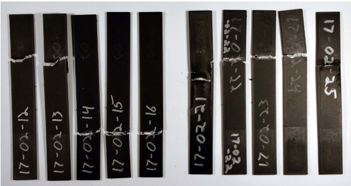
Figure A-8. Photo of the ASTM D3039 tensile failures in the Onyx/glass fiber series
