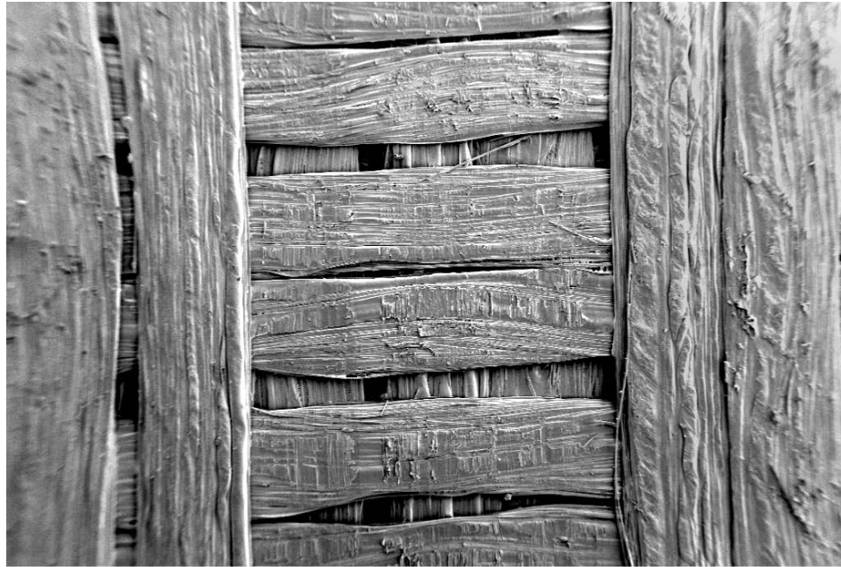
Figure A-9. Scanning electron micrograph of Onyx/glass fiber failure surface. The lack of fusion from filament to filament produced through-thickness pores.
