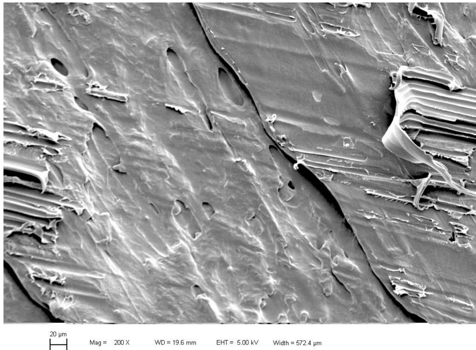
Figure A-11. Scanning electron micrograph of Onyx/glass fiber tensile failure surface. Delamination surface shows clean underlying ply with little adhesion from the removed ply.
