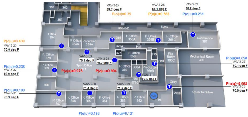
Figure 6. Floor plan showing thermostat locations in the administrative department and their probabilistic relationship to water dispenser (wd) usage.
