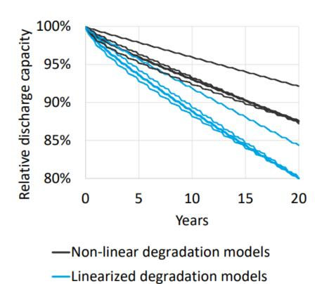
Linearized degradation model overestimates degradation, variance in degradation observed across different battery chemistry types is preserved.
