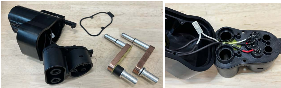
Figure 2. A disassembled J3400-to-CCS adapter
