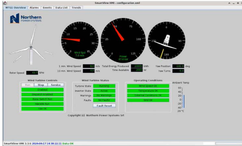
Figure 11. NPS SmartView showing a snapshot of wind turbine status. Image from Northern Power Systems
