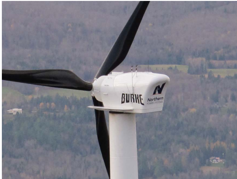
Figure 10. Nacelle-mounted anemometers and wind vanes provide input on inflow conditions to the turbine control system, such as on this NPS100 turbine. Photo from Chris Connor, Northern Power Systems
