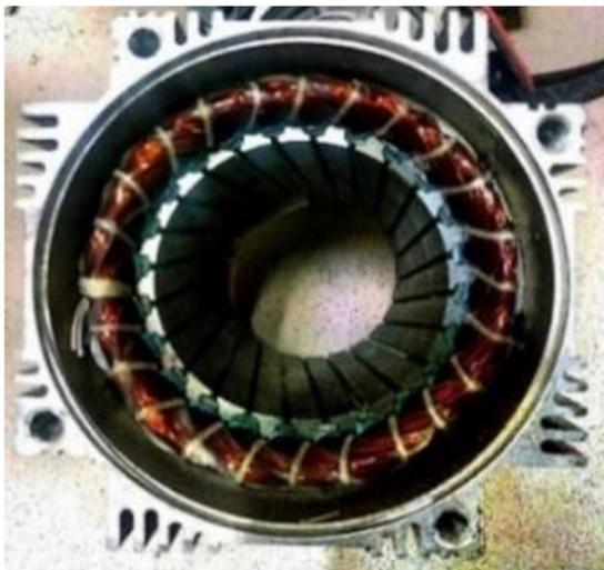
24-stator slot PM AC motor
