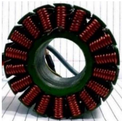
18-stator slot PM AC motor
