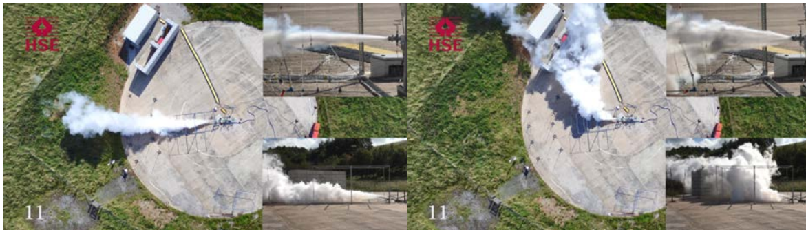
Figure 1: Stills from video taken during dispersion test 11 showing co-flow (left) and cross-flow (right) wind conditions
