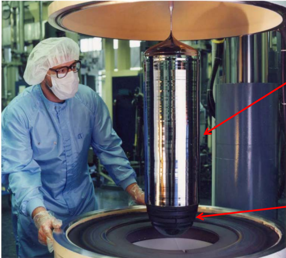
Fig. 1.2: Photograph of a silicon CZ puller with 200 mm crystal (Wacker Siltronic AG).
