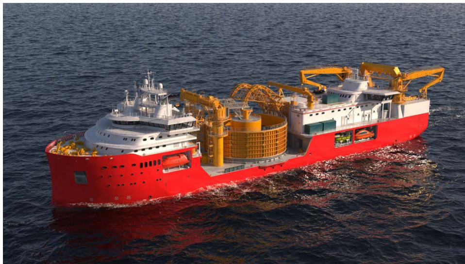
Figure 47. This visualization depicts a cable-laying vessel, which would be used to install transmission cables for offshore wind energy projects. Image from Josh Bauer, NREL
