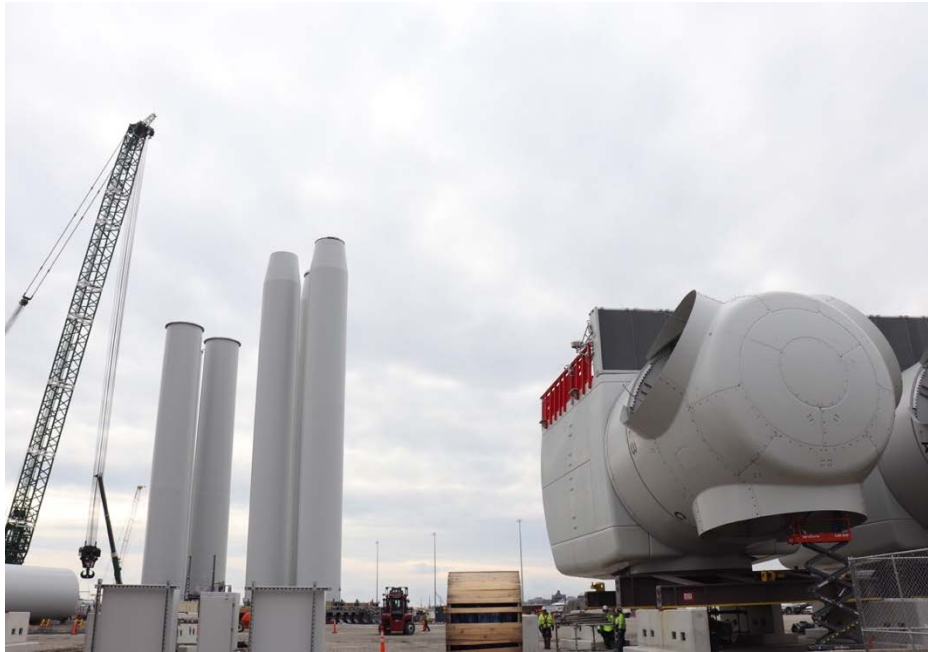
Figure 31. Components for the South Fork Wind project await transportation at State Pier in New London, Connecticut. State Pier was redeveloped to have offshore wind marshaling capabilities through a partnership between the state government and the South Fork Wind project developers. Photo from Matilda Kreider, NREL
