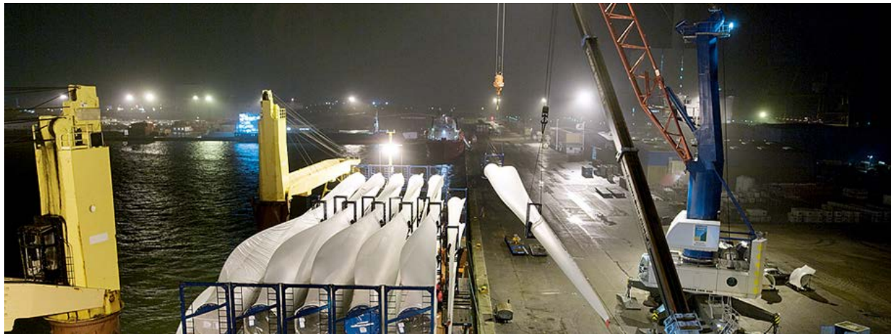
Figure 18. At a port in Denmark, blades are loaded onto a vessel to be transported to an offshore wind energy project site. Photo from Siemens AG 27843
