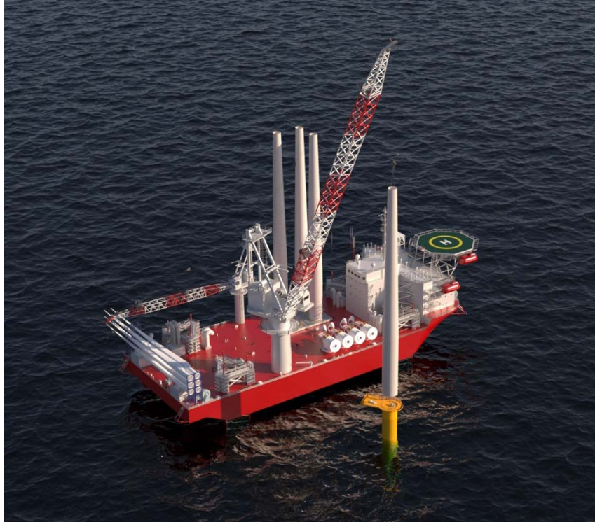
Figure 46. This visualization depicts a wind turbine installation vessel installing a turbine. Image from Josh Bauer, NREL
