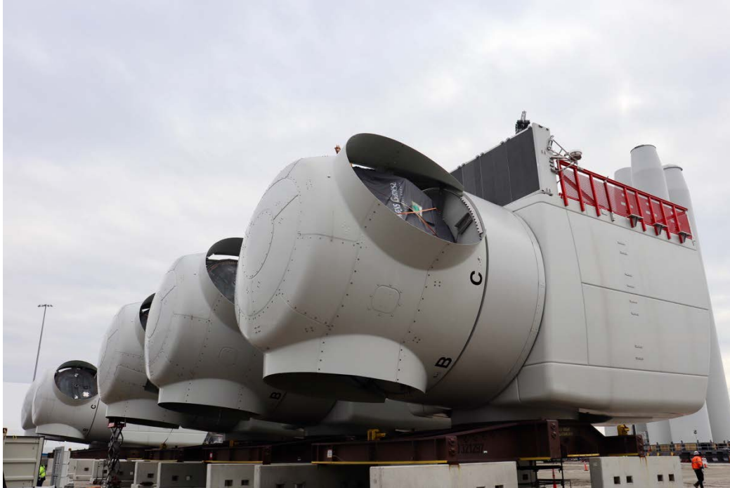
Figure 6. Nacelles for the South Fork Wind project await transportation at State Pier in New London, Connecticut. Photo from Matilda Kreider, NREL
